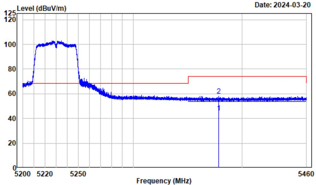
**802.11ac40**Test Channel: **5230MHz** Ant. Polar. : **Vertical**
