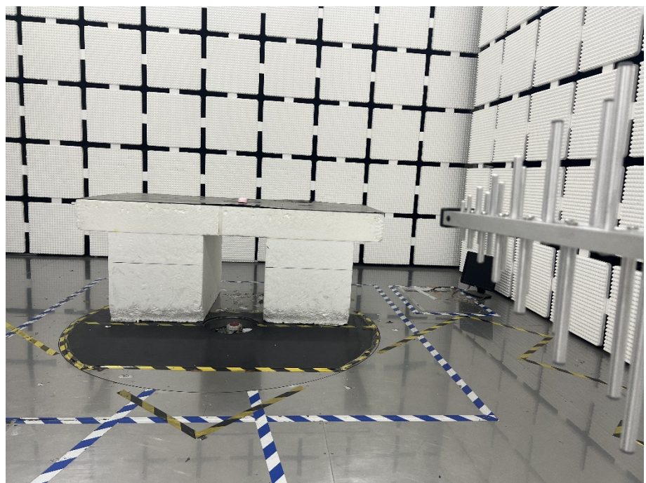
Radiation Emission Test Setup (30MHz to 1GHz)
