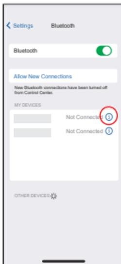
14. Click “Forget This Device” to remove the Transformer from the bluetooth device list.
