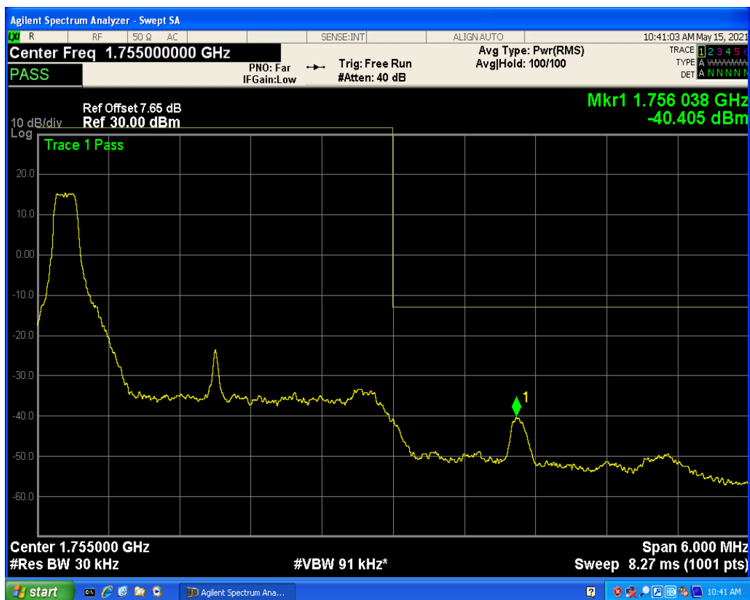
Band4 QAM16 BW=3MHz Channel=20385 RB Size=15 Position=#0
