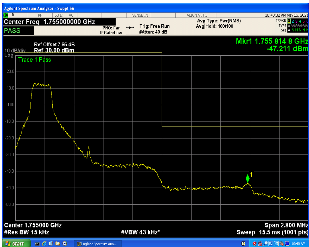
Band4 QAM16 BW=1.4MHz Channel=20393 RB Size=6 Position=#0
