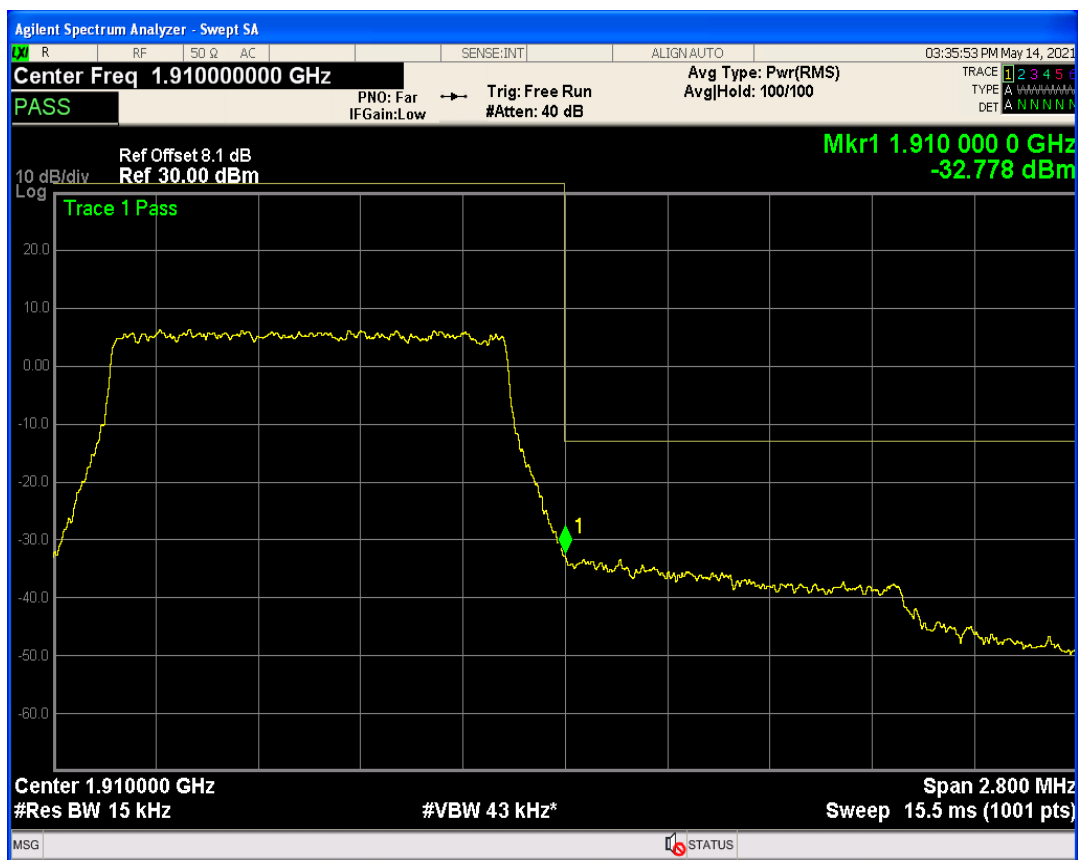
Band2 QAM16 BW=1.4MHz Channel=19193 RB Size=1 Position=#0
