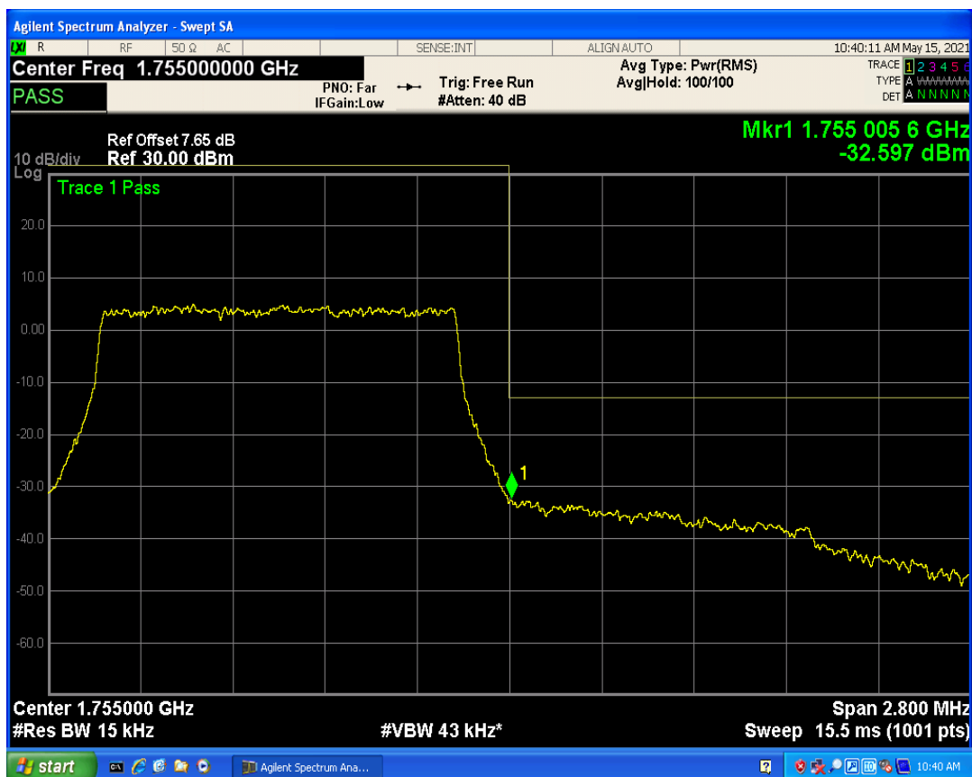
Band4 QAM16 BW=1.4MHz Channel=20393 RB Size=1 Position=#Max
