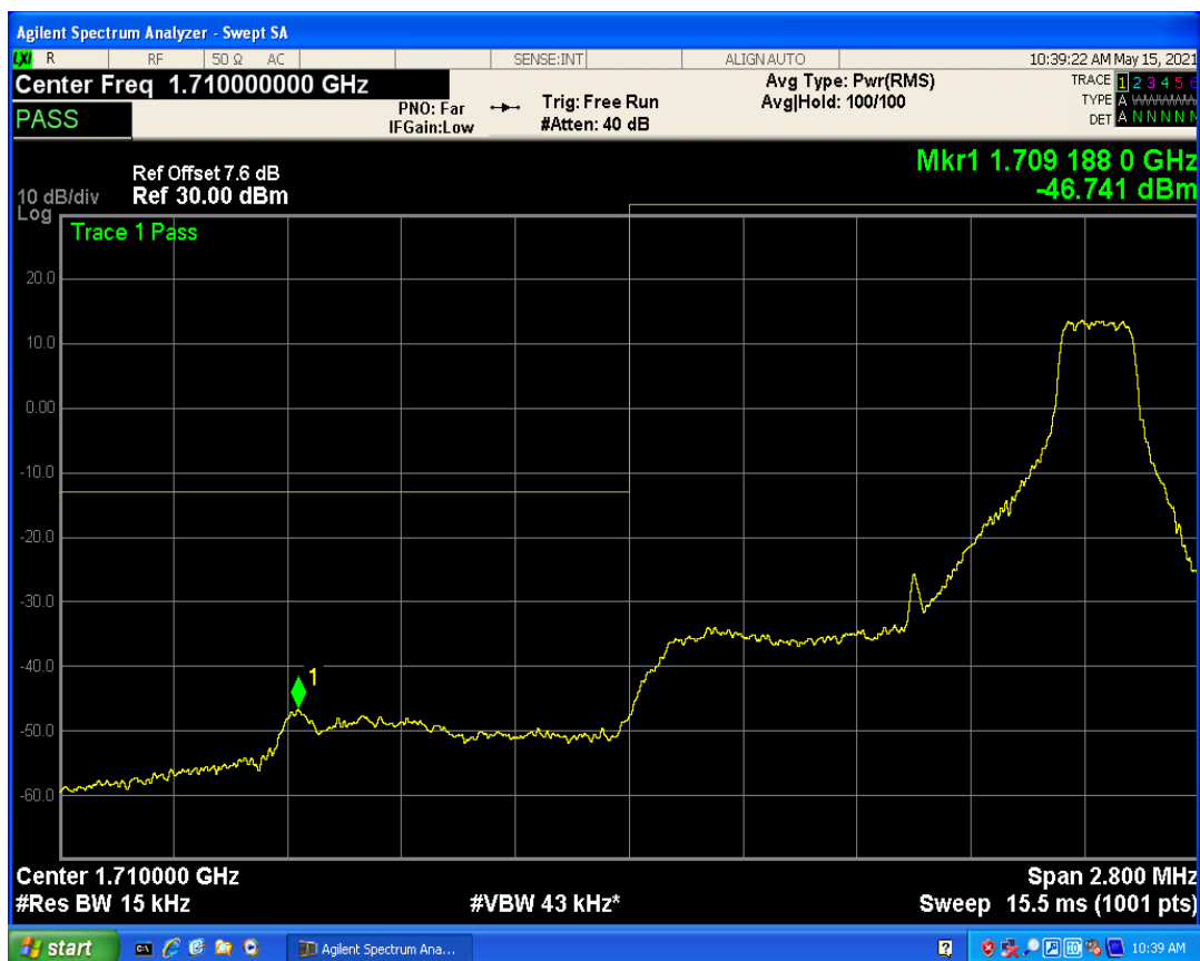
Band4 QPSK BW=1.4MHz Channel=19957 RB Size=6 Position=#0
