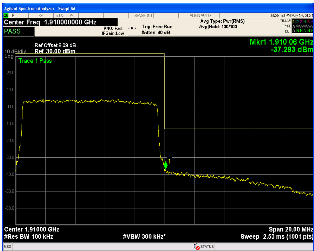
Band2 QPSK BW=15MHz Channel=18675 RB Size=75 Position=#0
