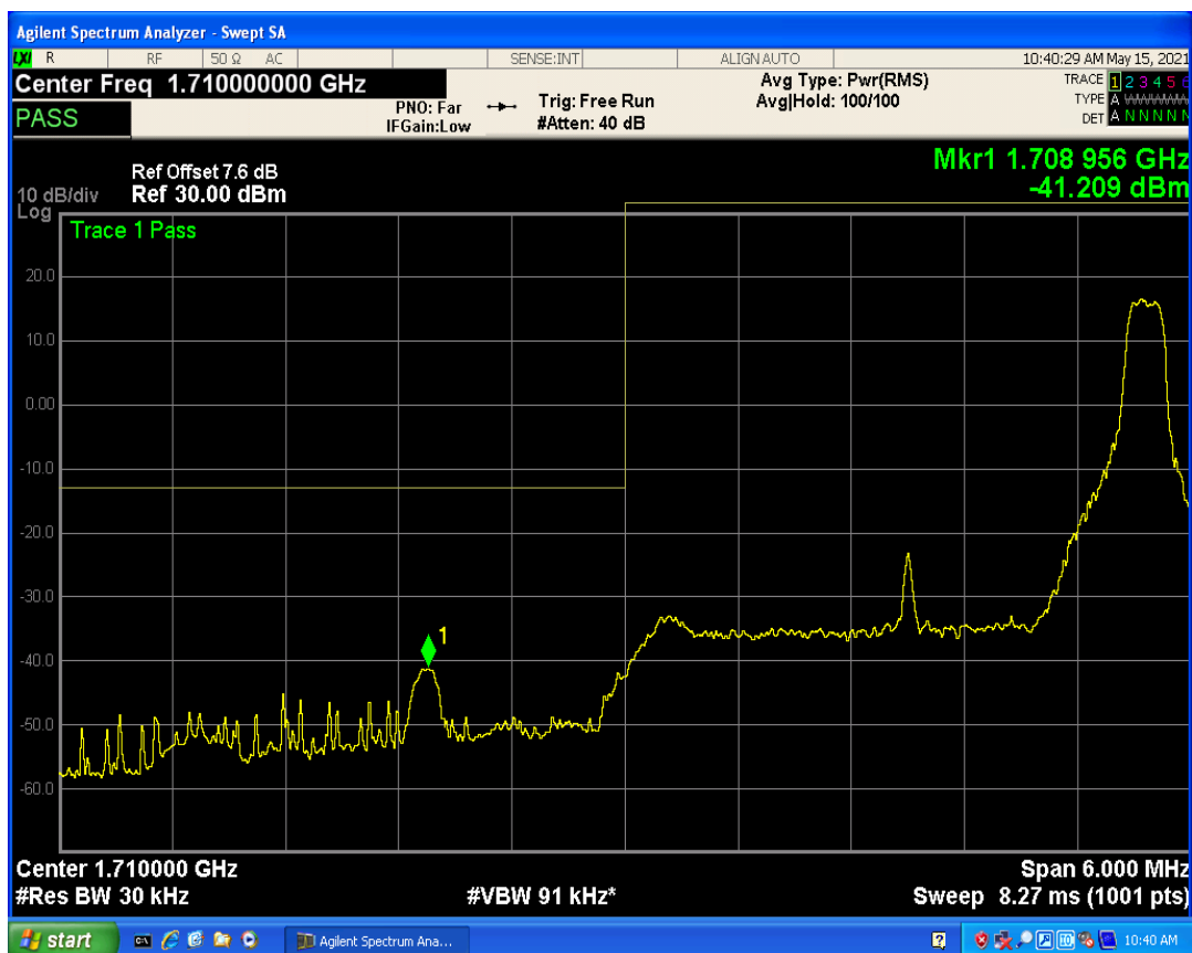
Band4 QAM16 BW=3MHz Channel=19965 RB Size=1 Position=#0
