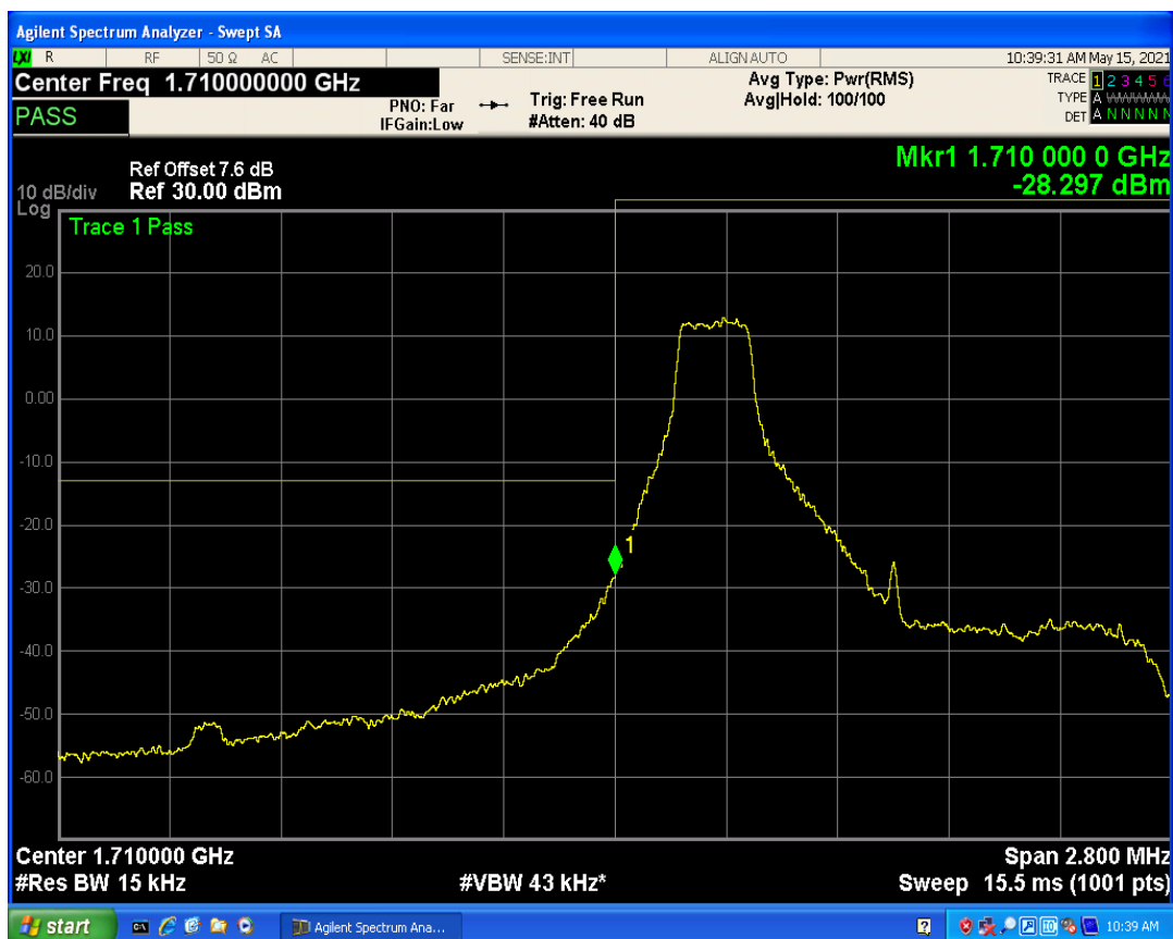
Band4 QAM16 BW=1.4MHz Channel=19957 RB Size=6 Position=#0
