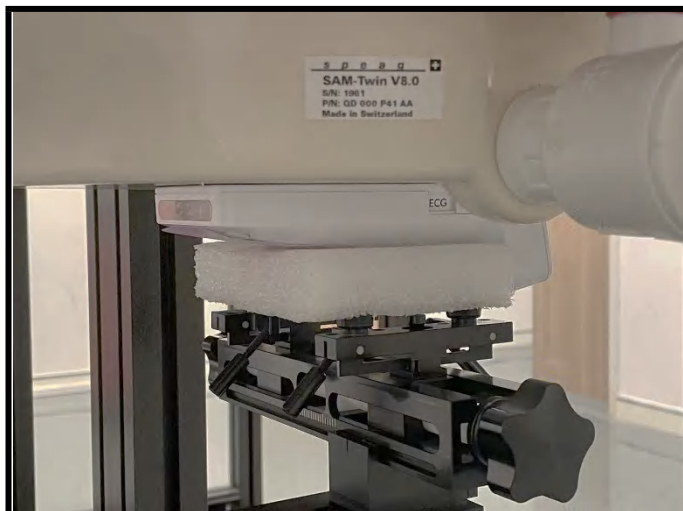
Front Face of EUT with 0 cm Gap
