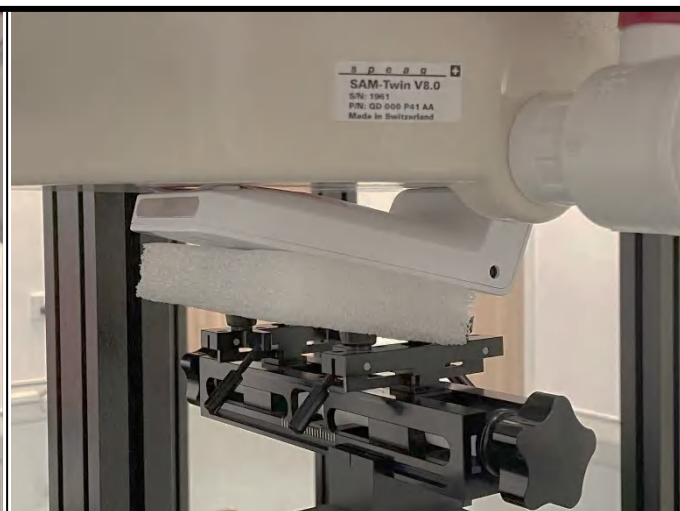
Rear Face of EUT with 0 cm Gap
