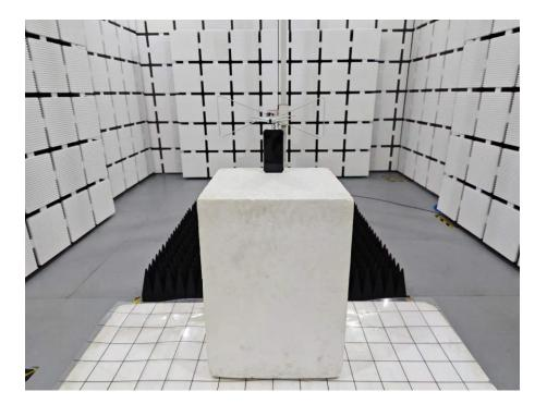
Set-up for Transmitter & Receiver Spurious Emissions, Below 1GHz
