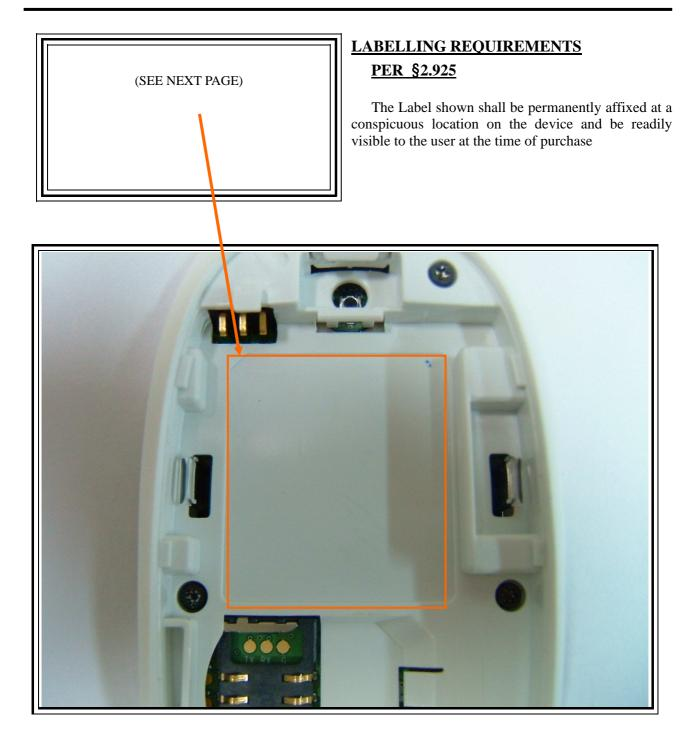
Note: 1. The label generally is located underneath a back door of the phone.
