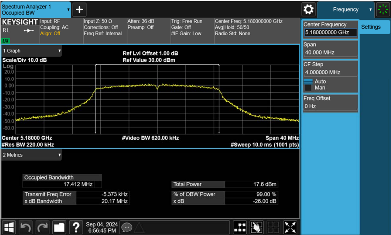
Figure 4: 802.11n(HT20), 5180MHz Test Plot of -26dB Bandwidth and 99% Bandwidth
