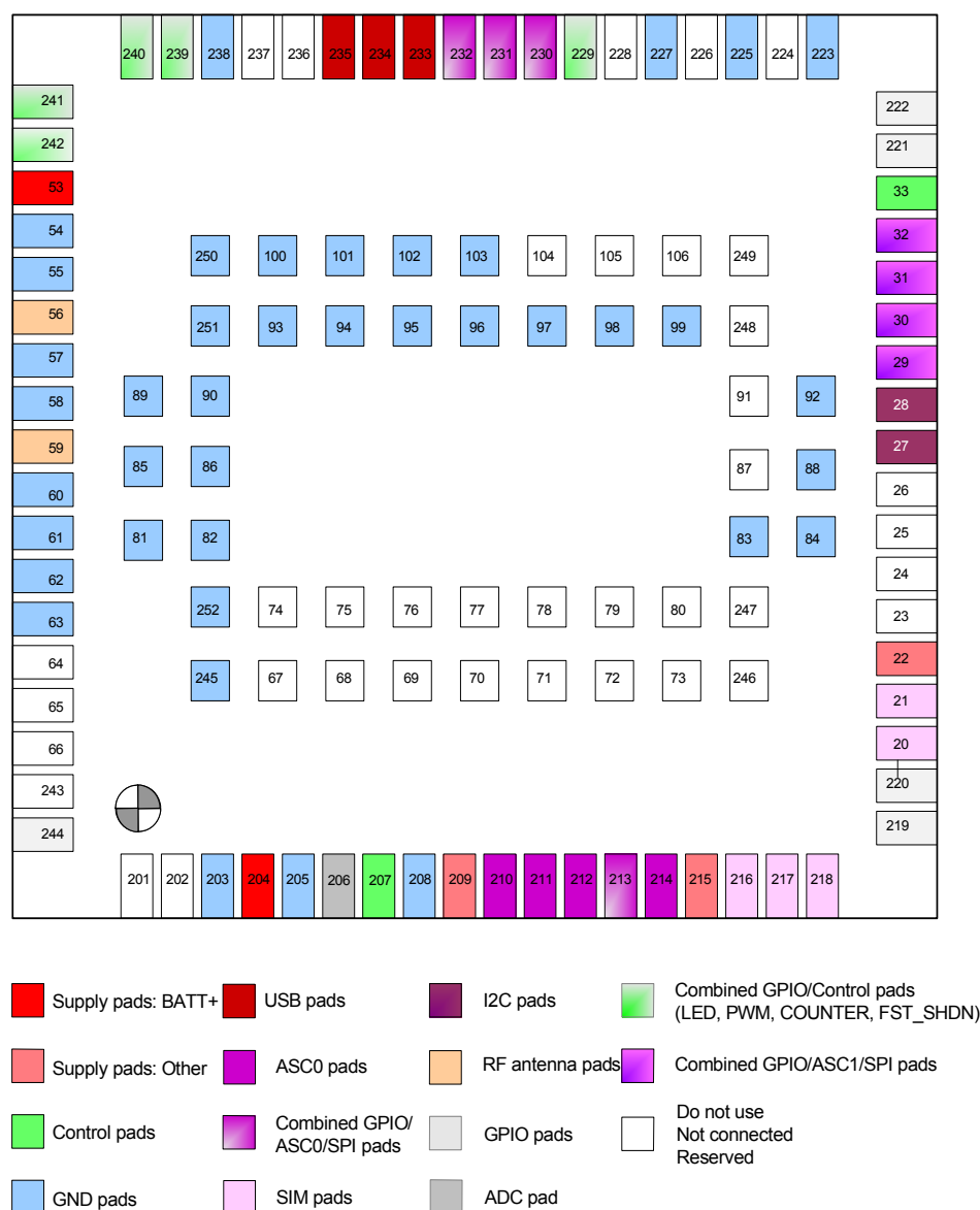
Figure 4: Numbering plan for connecting pads (bottom view)
