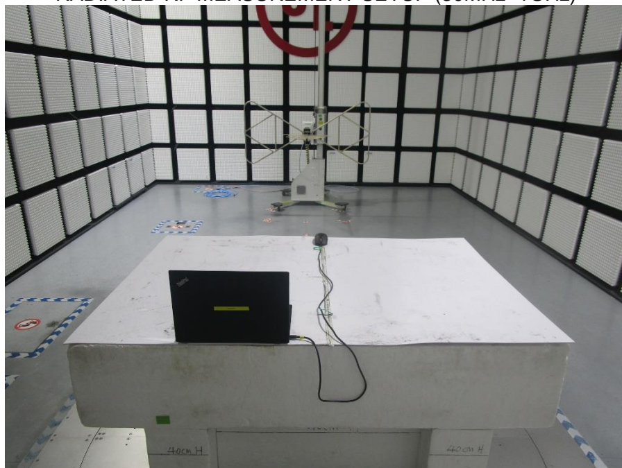
RADIATED RF MEASUREMENT SETUP (Below 30MHz)
