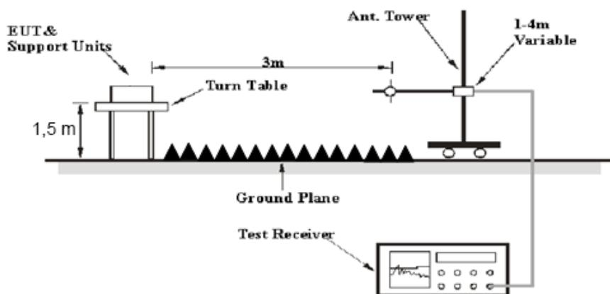
The radiated emission below 1GHz tests were performed in the 10 meters chamber test site, above 1GHz tests were performed in the 3 meters chamber test site A, using the setup accordance with the ANSI C63.10-2013. The specification used was the FCC 15.209, and FCC 15.247 limits and the RSS-247 Clause 5.5, RSS-GEN Clause 8.10 limits.
