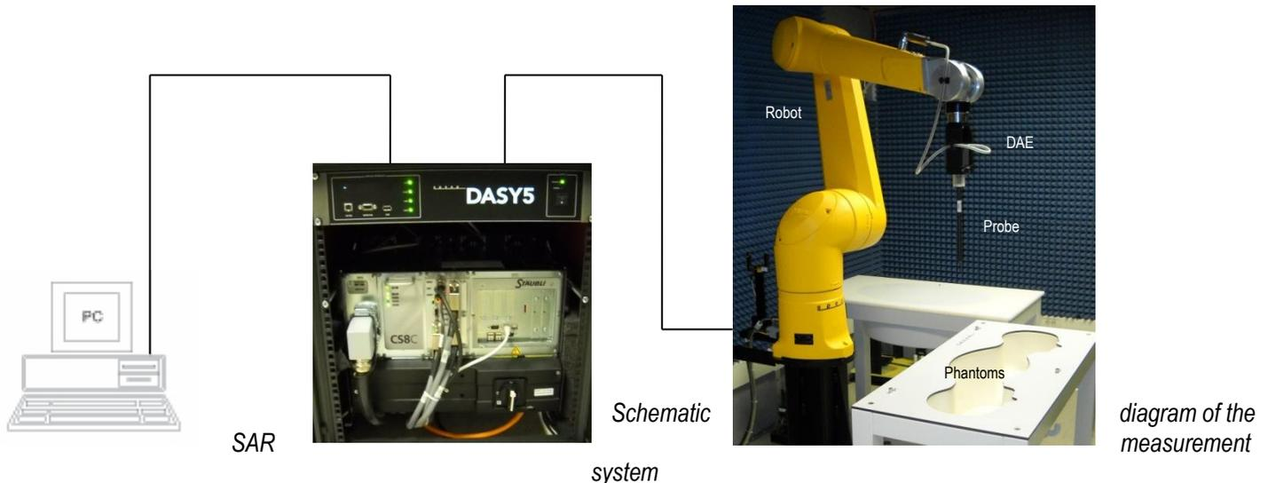
In operation, the system first does an area (2D) scan at a fixed depth within the liquid from the inside wall of the phantom. When the maximum SAR point has been found, the system will then carry out a 3D scan centered at that point to determine volume averaged SAR level.
