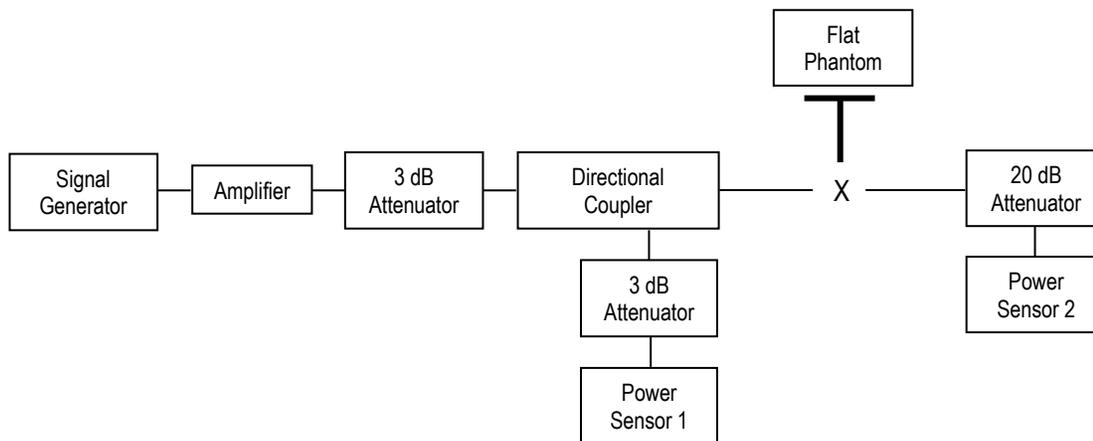
1. The cable at the output of the directional coupler is connected to the 20 dB attenuator.
