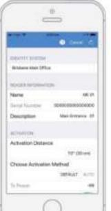
Select the corresponding IDENTITY SYSTEM from the drop down box. Assign a short "Name" and "Description" using alphanumeric characters. Enable the slider for "Self Enrollment" if you intend to allow your users to enroll mobile credential using their existing legacy cards from this reader. Click 'Save' to successfully complete reader configuration.
