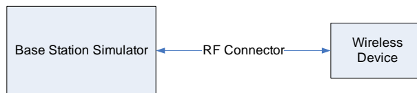
Figure 9-1 Power Measurement Setup
