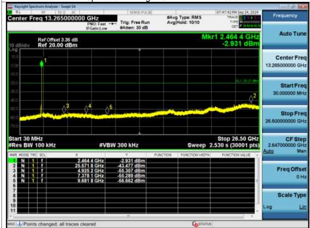
Tx. Spurious NVNT g 2462MHz Ant1 Emission
