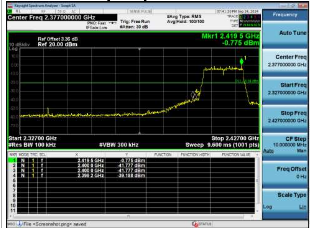
Band Edge NVNT g 2412MHz Ant1 Emission
