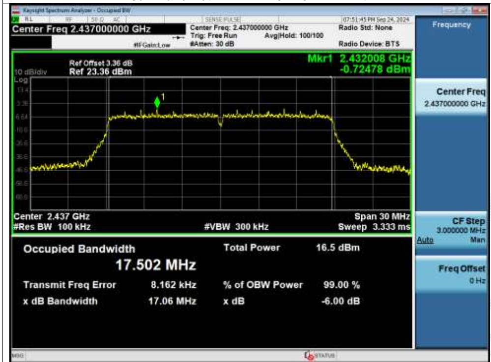
-6dB Bandwidth NVNT n20 2437MHz Ant1
