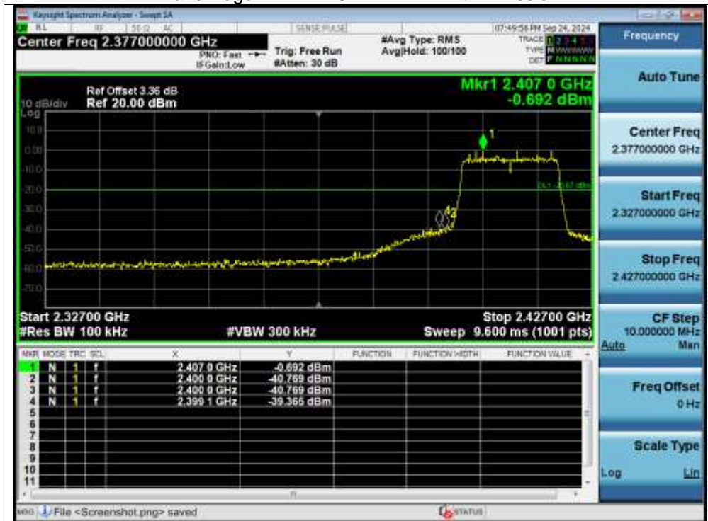
Band Edge NVNT n20 2412MHz Ant1 Emission
