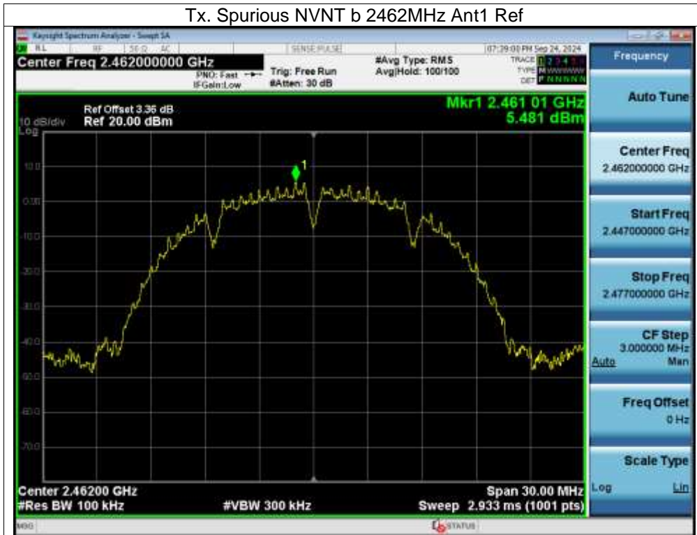
Tx. Spurious NVNT b 2462MHz Ant1 Emission
