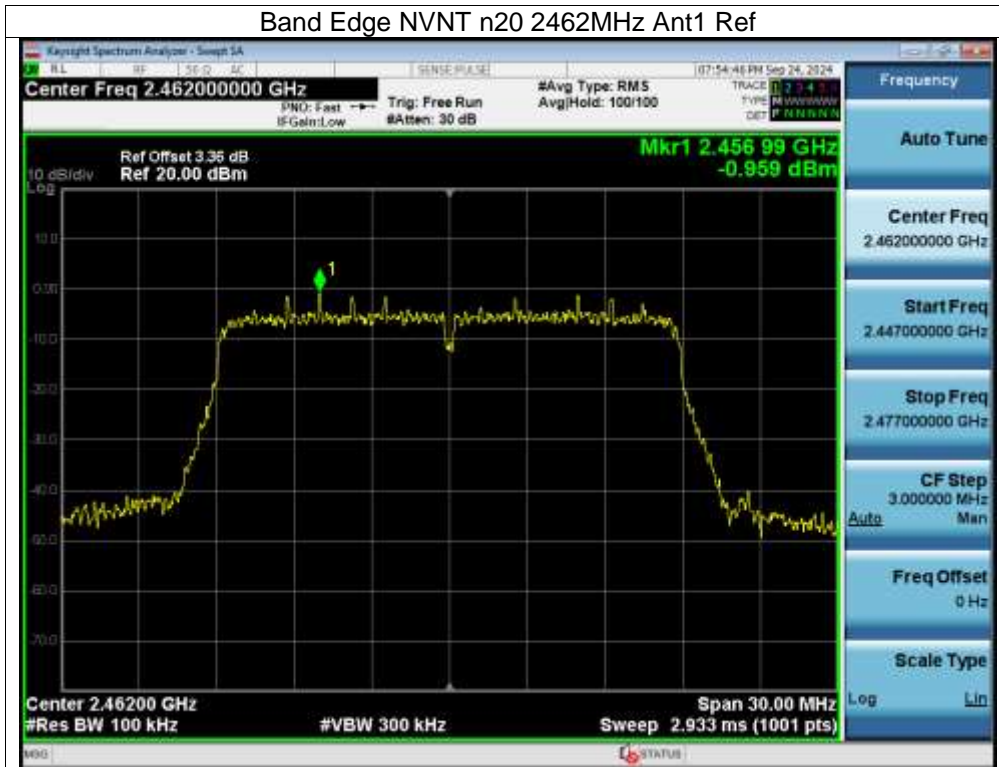
Band Edge NVNT n20 2462MHz Ant1 Emission
