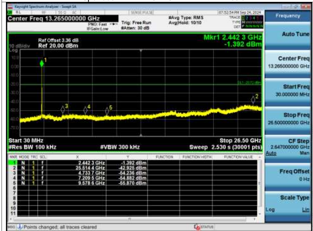
Tx. Spurious NVNT n20 2437MHz Ant1 Emission
