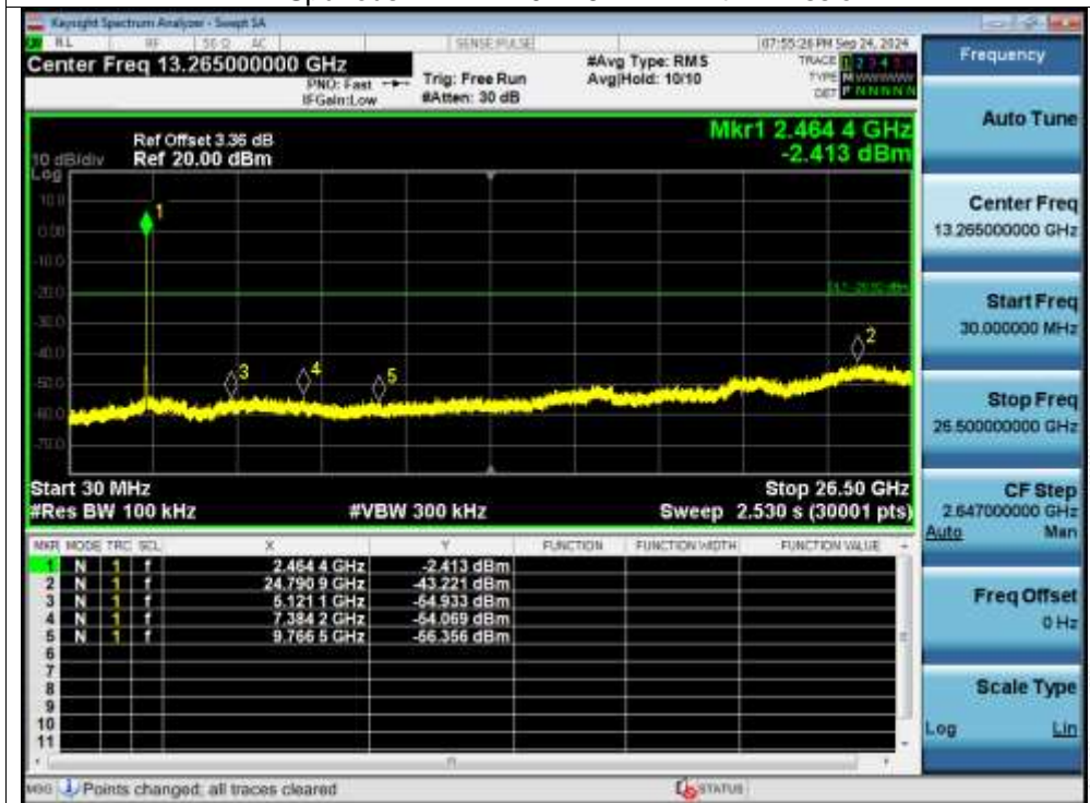
Tx. Spurious NVNT n20 2462MHz Ant1 Emission
