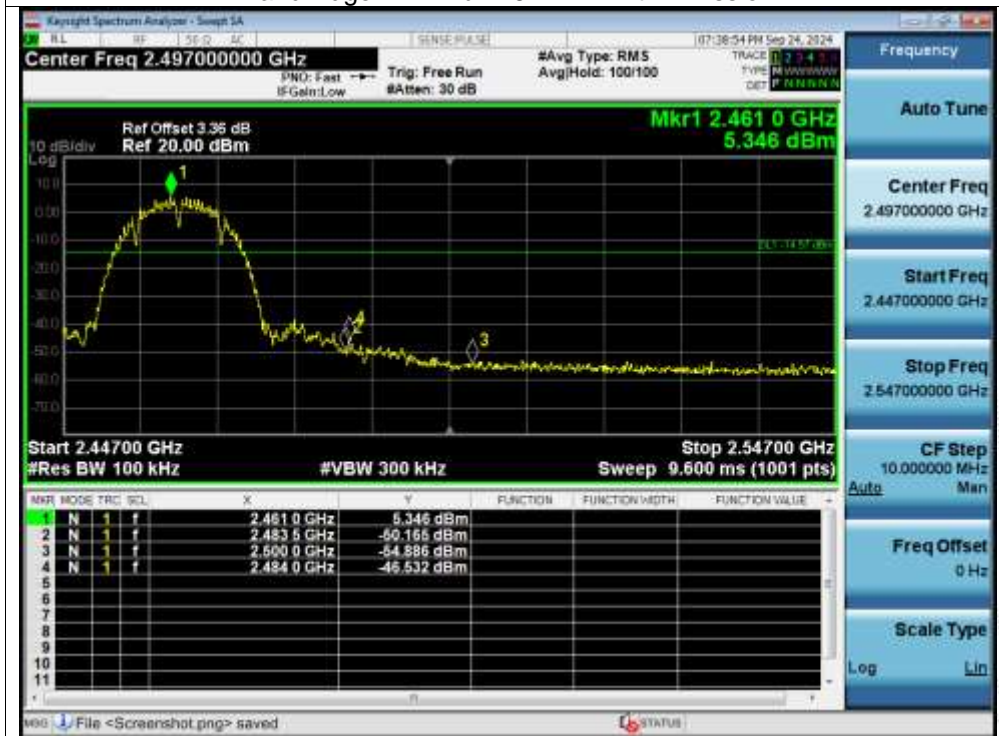
Band Edge NVNT b 2462MHz Ant1 Emission
