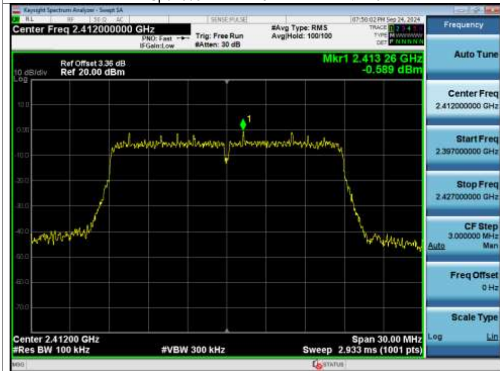
Tx. Spurious NVNT n20 2412MHz Ant1 Emission
