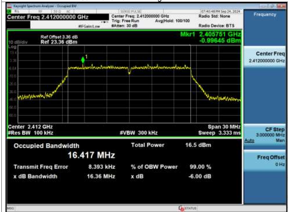
-6dB Bandwidth NVNT g 2412MHz Ant1
