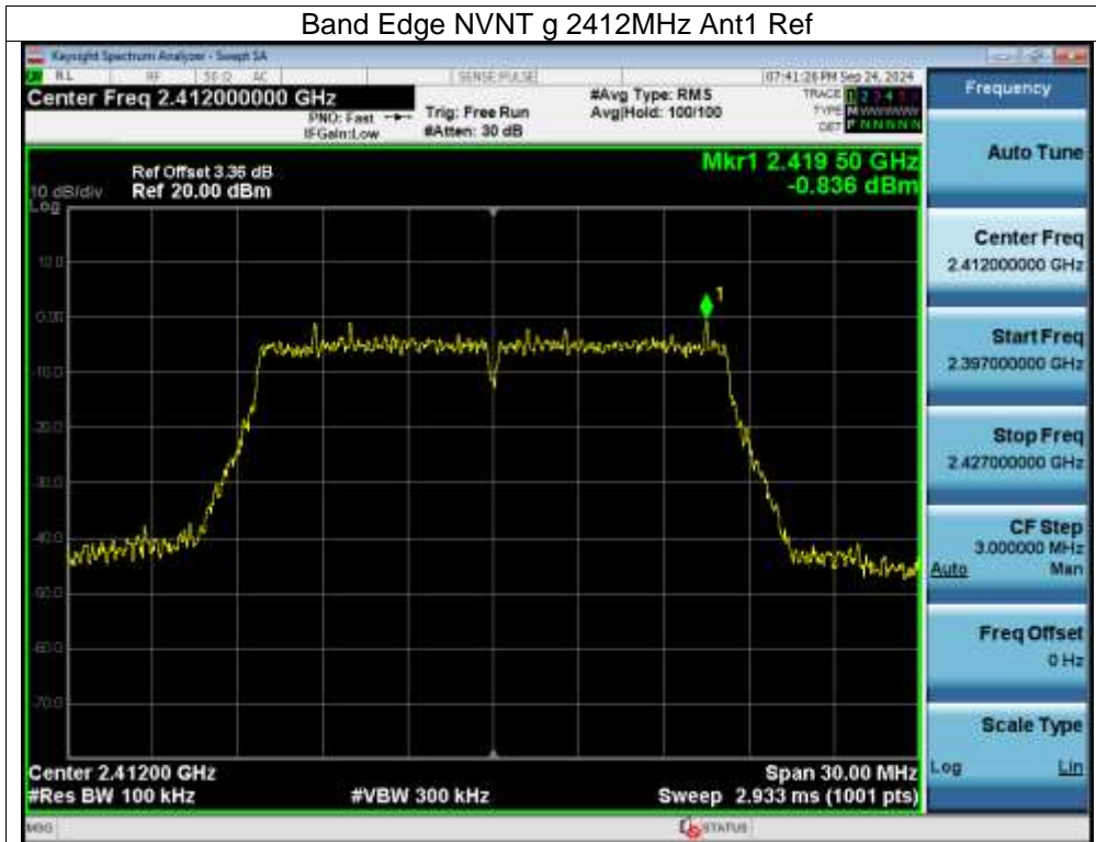
Band Edge NVNT g 2412MHz Ant1 Emission
