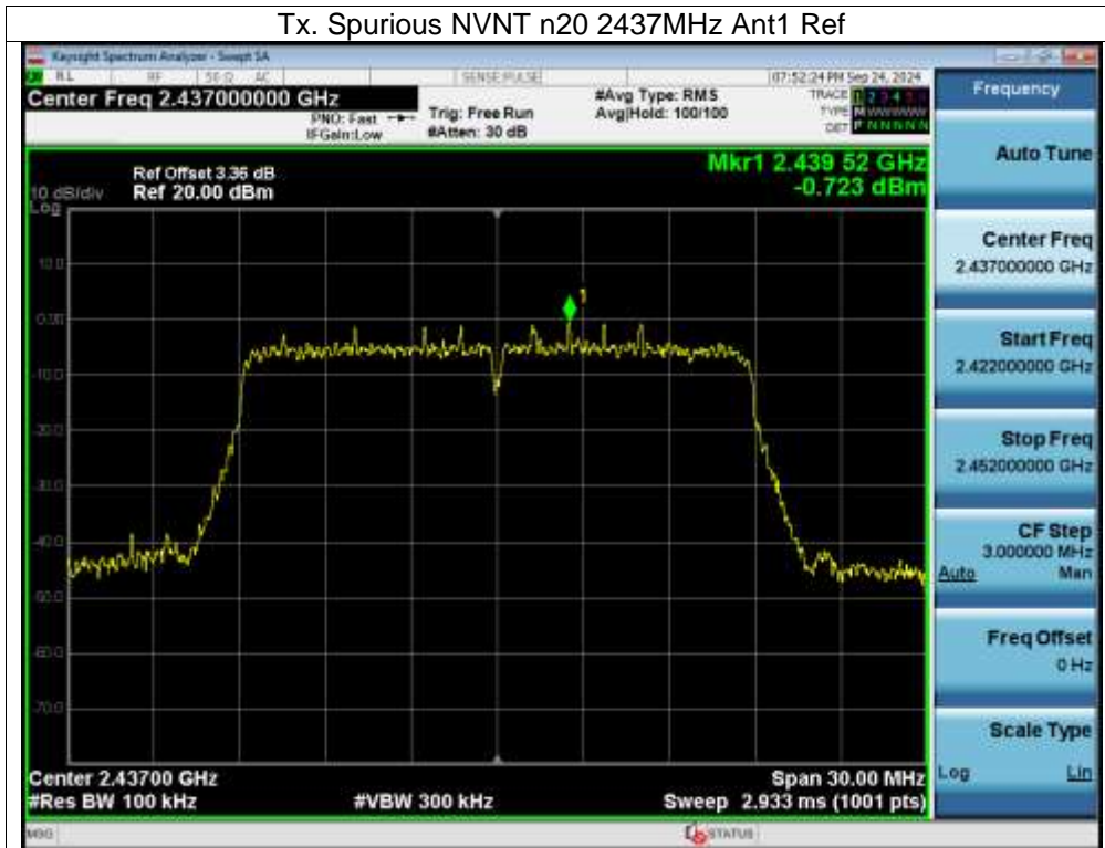
Tx. Spurious NVNT n20 2437MHz Ant1 Emission
