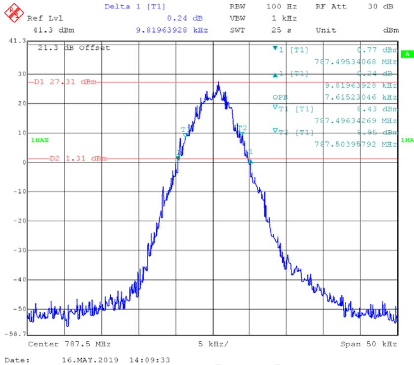
**4FSK,12.5kHz,Low Power - Frequency 453.2125MHz: 99% Occupied & 26 dB Bandwidth**
