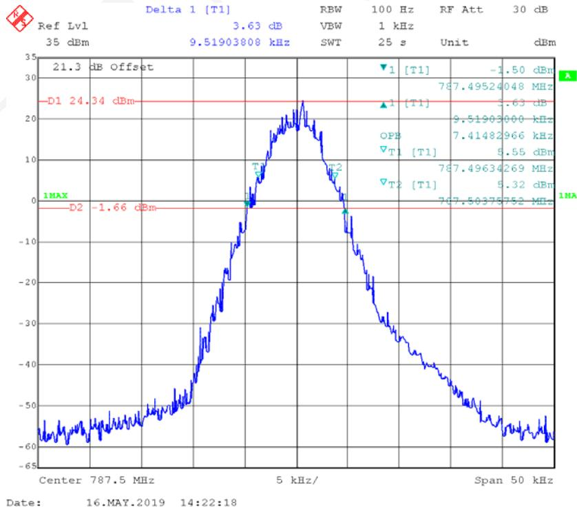
**FFSK/1200,12.5kHz,High Power - Frequency 787.5MHz: 99% Occupied & 26 dB Bandwidth**
