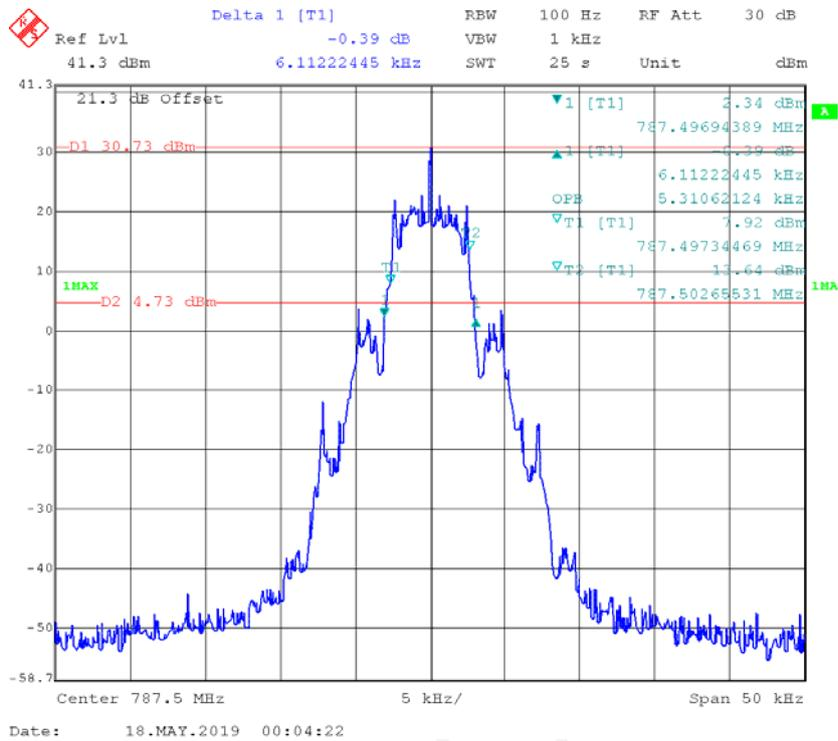
**FFSK/2400,12.5kHz,Low Power - Frequency 787.5MHz: 99% Occupied & 26 dB Bandwidth**
