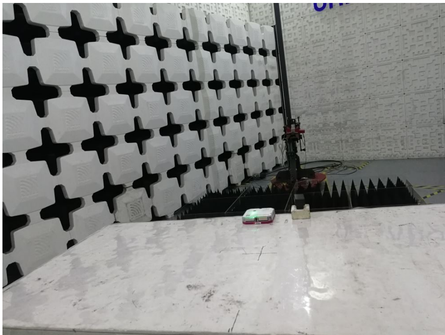
Photograph 2: Set-up for Radiated Emission, above 1GHz
