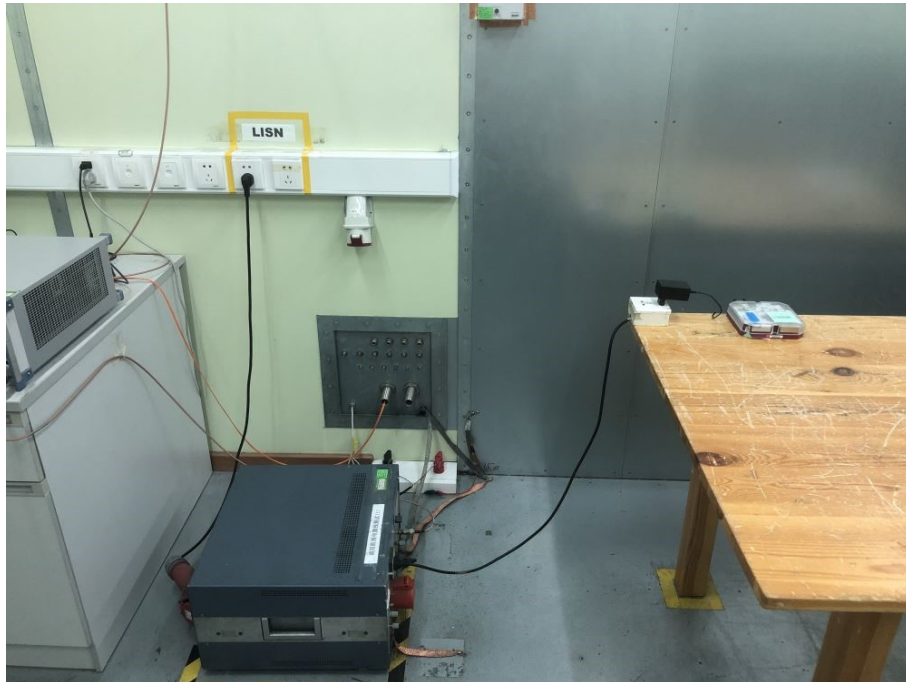
Photograph 3: Set-up for Conducted Emission on AC Main
