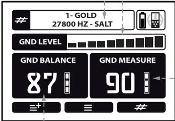
The image shows the LCD screen of the SOL detector. At the top, it displays "# 1- GOLD 27800 HZ - SALT" and a battery level indicator. Below this is a "GND LEVEL" bargraph. The screen is split into two main sections: "GND BALANCE" showing a large number "87" and "GND MEASURE" showing a large number "90". At the bottom, there are three buttons: a left arrow, a right arrow, and a "#". Dashed lines connect these elements to the text on the right.
