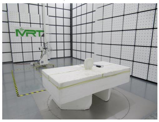
Description: Radiated Spurious Emission Test Setup for above 1GHz (BLE & Scan Antenna & 5G Wi-Fi band1, 2)
