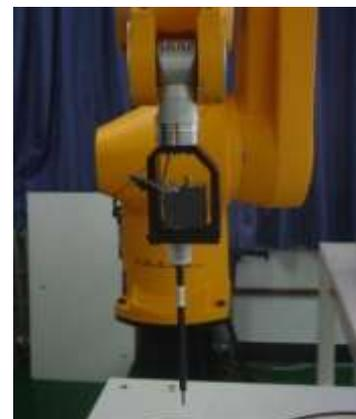
Picture C.3E-field Probe
