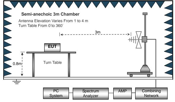
(C) Radiated Emission Test-Up Frequency Above 1GHz
