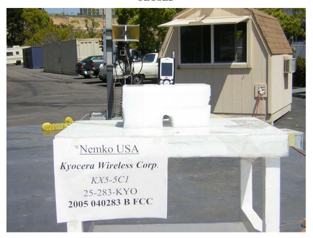
Photograph 2. FCC, Part 22/24 Radiated Substitution Emissions Test Configuration
