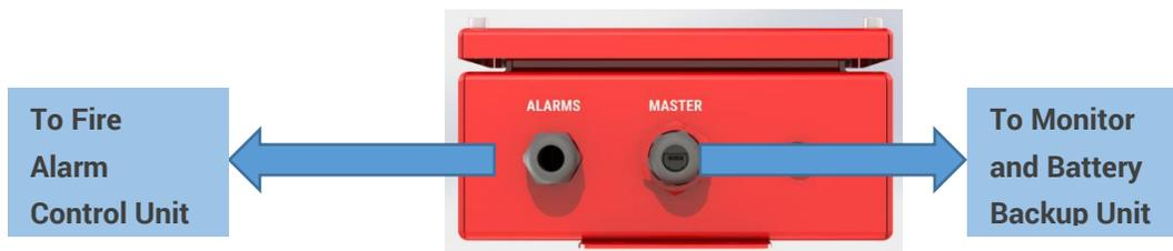
Figure 18. Remote Annunciator port layout
