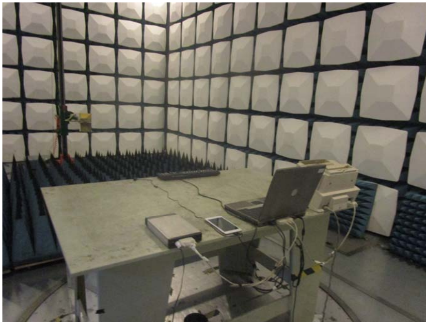
Radiated Emission Above 1GHz – Rear View
