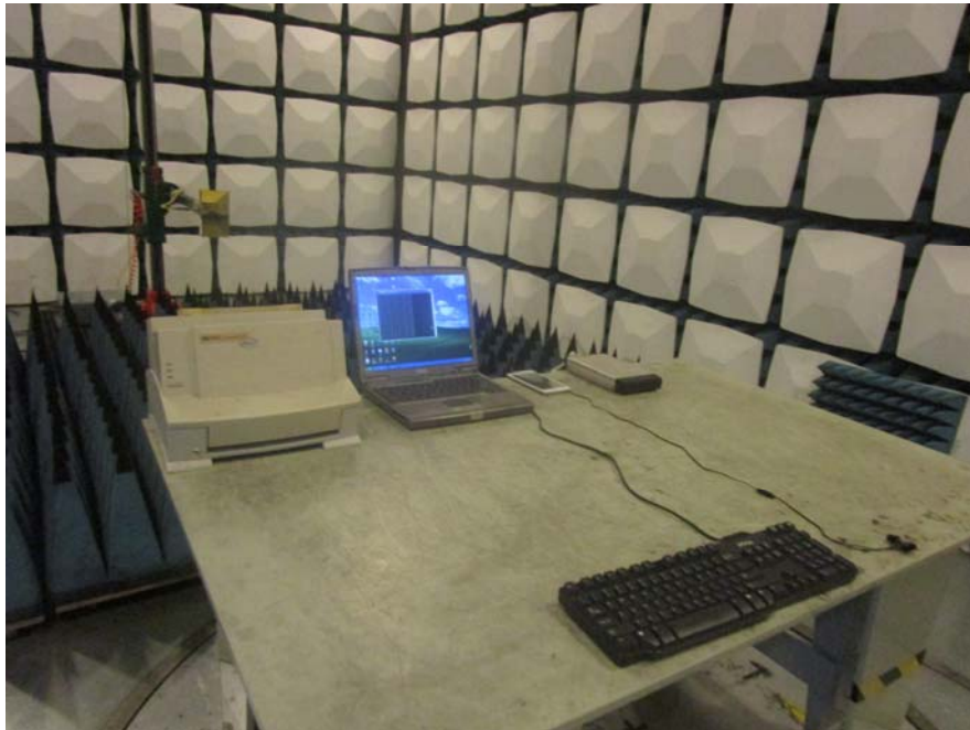
Radiated Emission Above 1GHz – Front View
