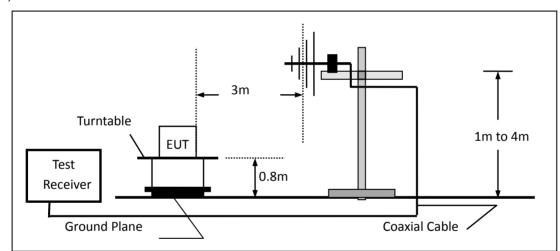
(c) For radiated emissions above 1000MHz
