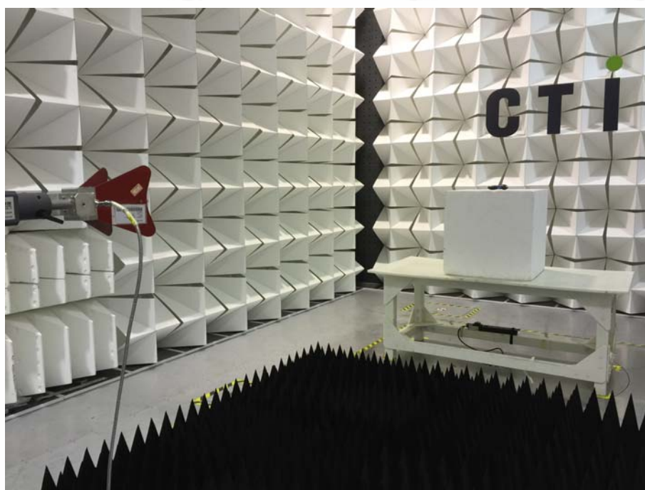
Radiated spurious emission Test Setup-2(Above 1GHz)
