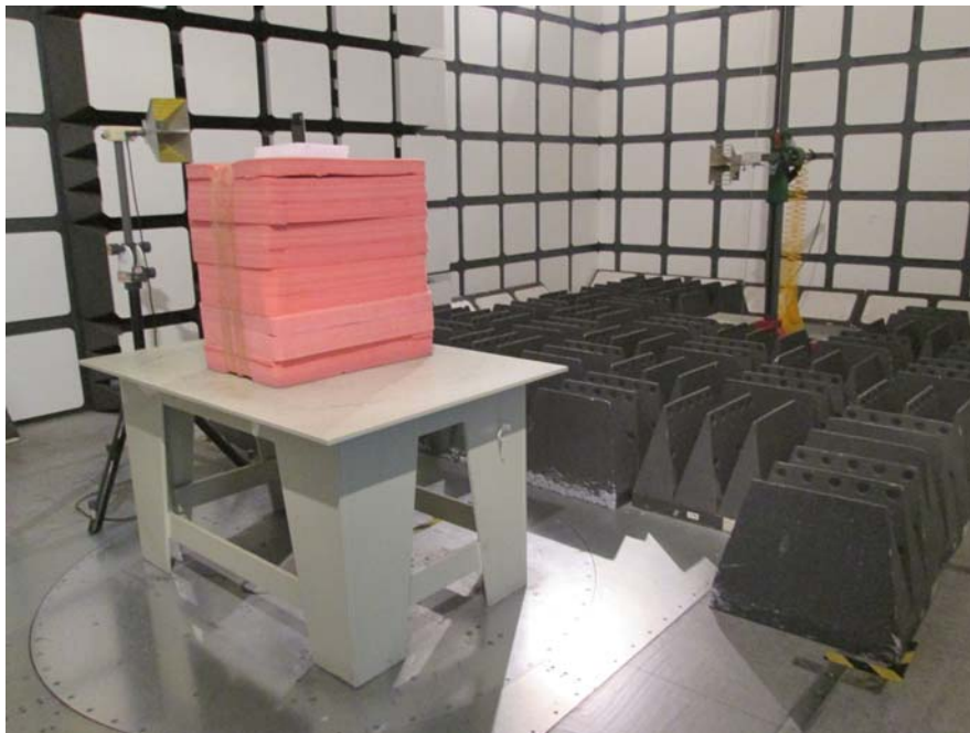
Radiated Emissions Test View (Above 1 GHz)
