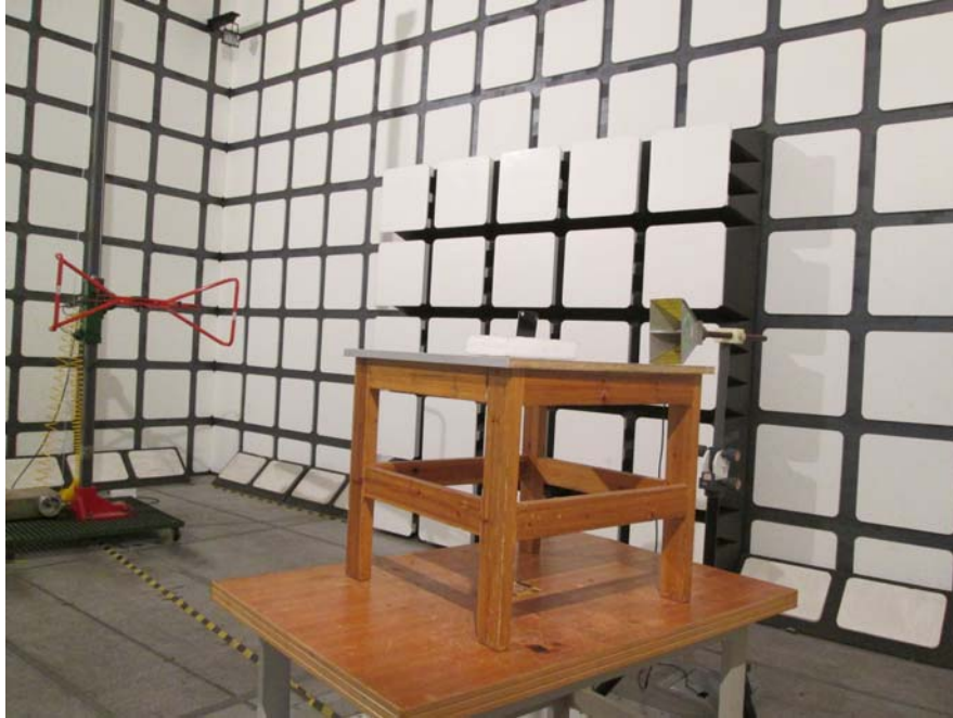
Radiated Emissions Test View (Below 1 GHz)
