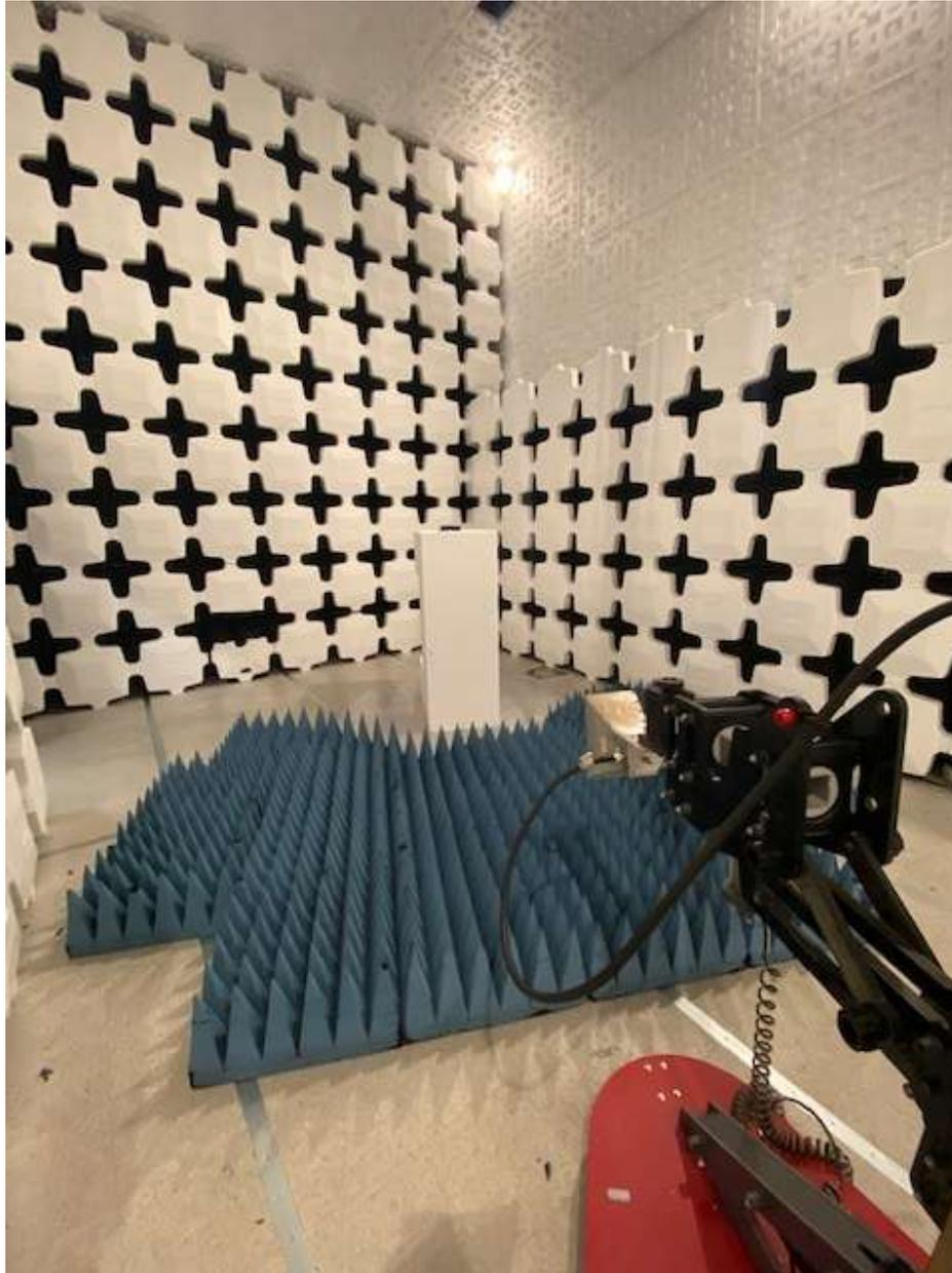
**Figure 4. Spurious Emissions Configuration (Above 1000 MHz)**
