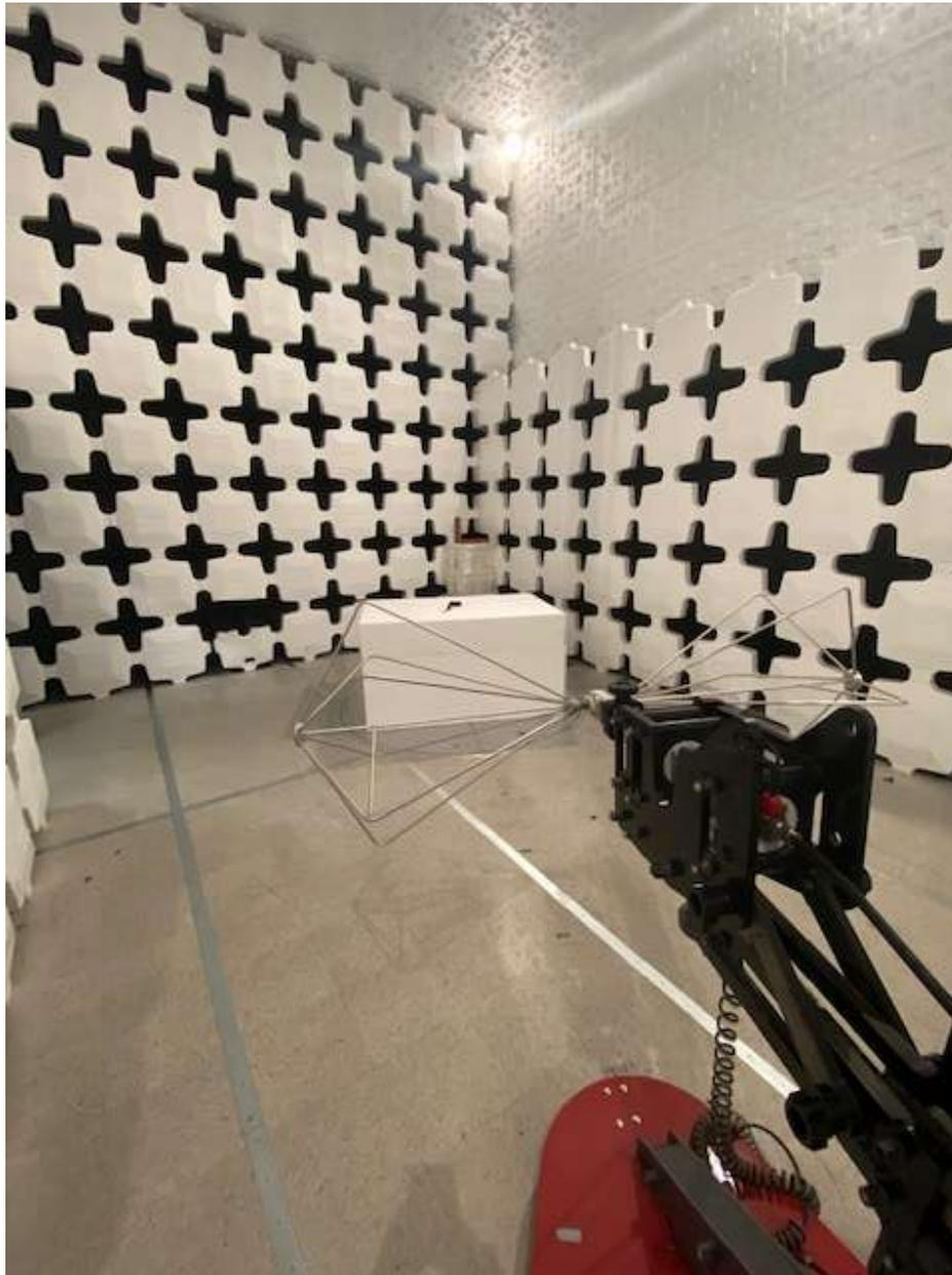
**Figure 2. Spurious Emissions Configuration (30 – 200 MHz)**
