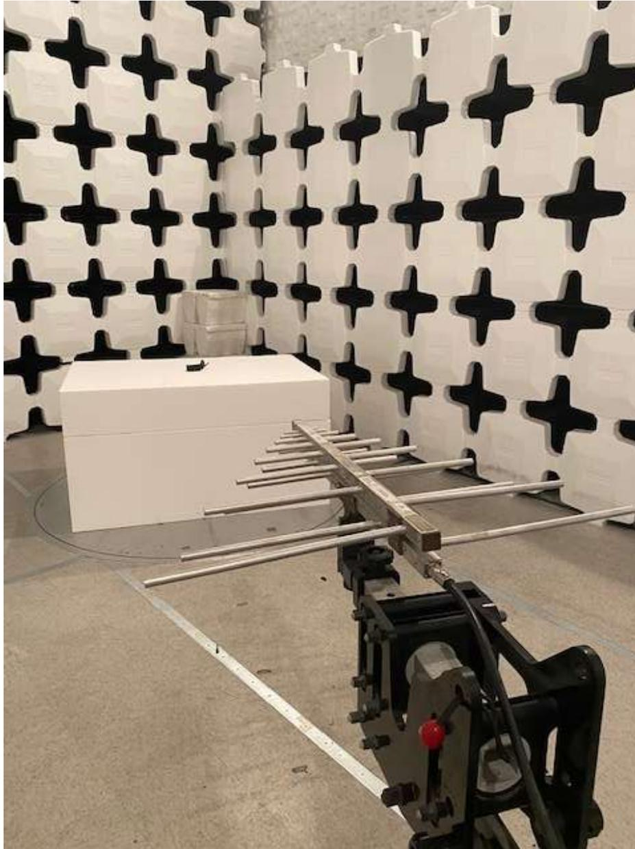
**Figure 3. Spurious Emissions Configuration (200 – 1000 MHz)**
