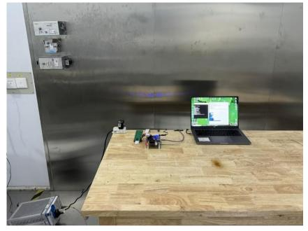
**RF Conducted Test Setup**
