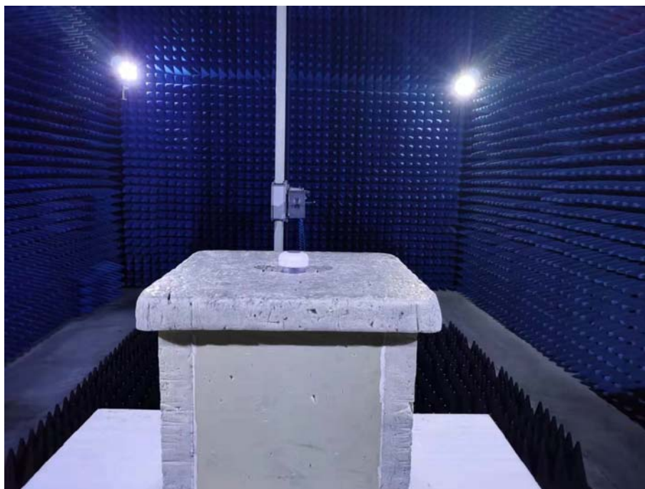
Photo of Radiated Emission Measurement Above 1GHz
