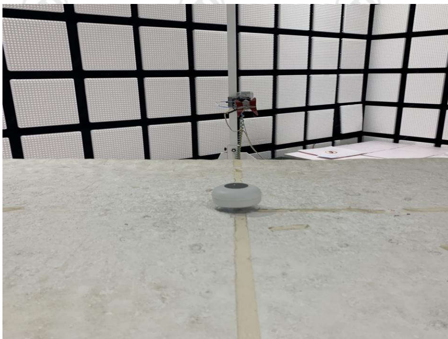
Radiated spurious emission Test Setup-2(Above 1GHz)
