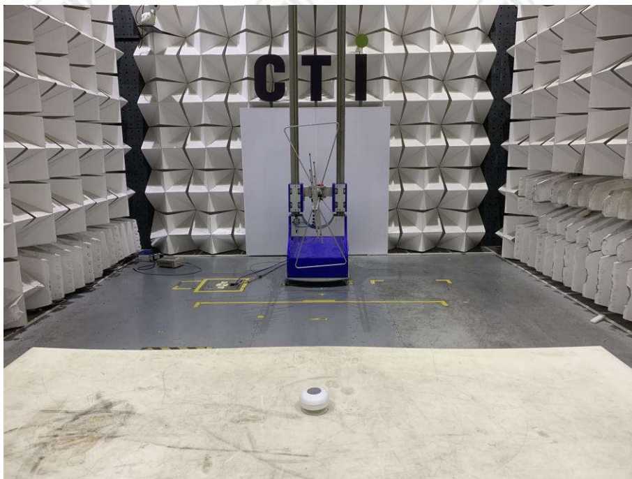
Radiated spurious emission Test Setup-1(Below 1GHz)
