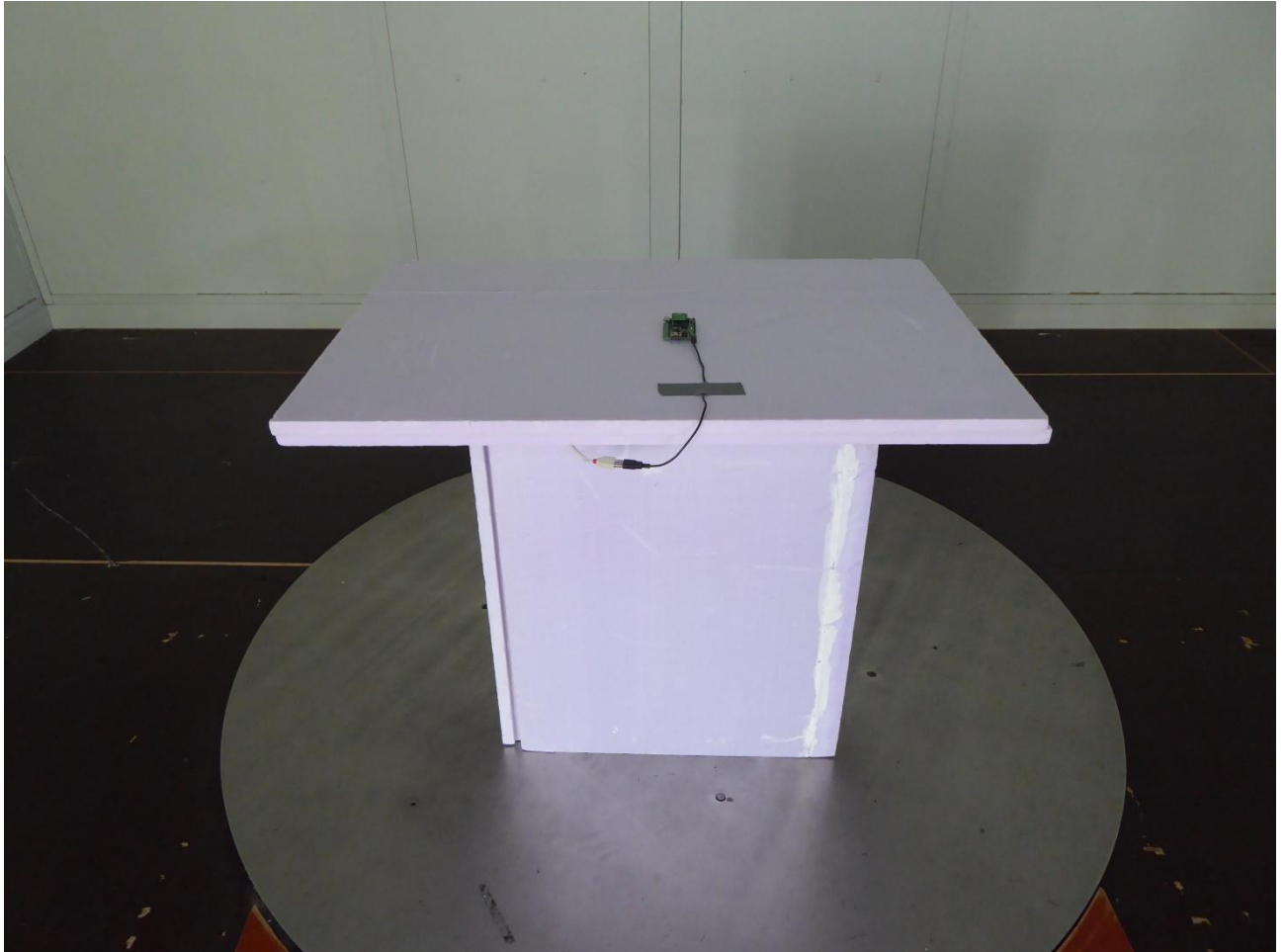
Test setup open area test site 30 MHz – 1 GHz
