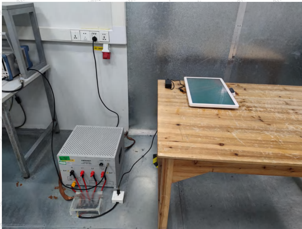
Photo of Conducted Emission Measurement
