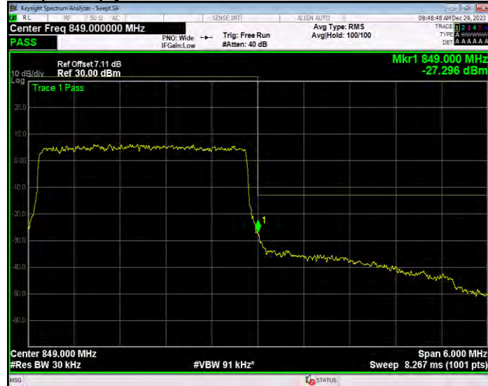
Band26(824-849) QPSK BW=5MHz Channel=26815 RB Size=25 Position=#0
