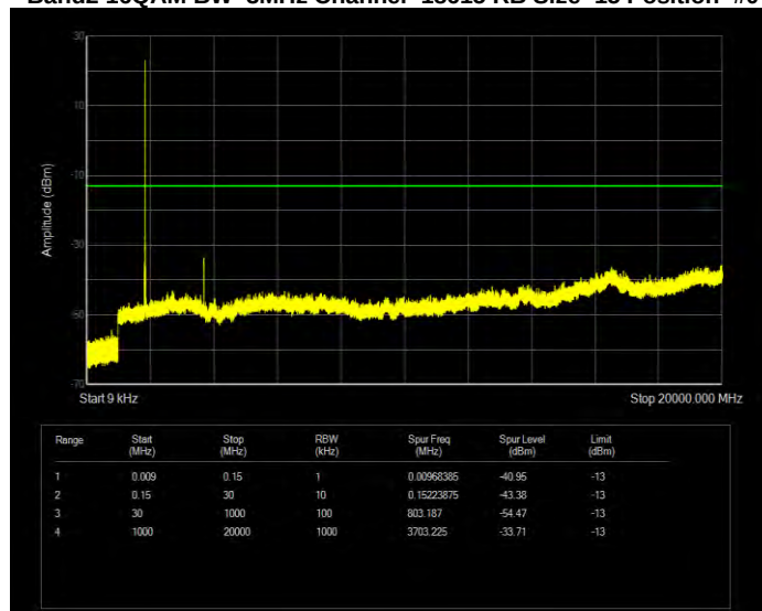
Band2 16QAM BW=3MHz Channel=18900 RB Size=15 Position=#0
