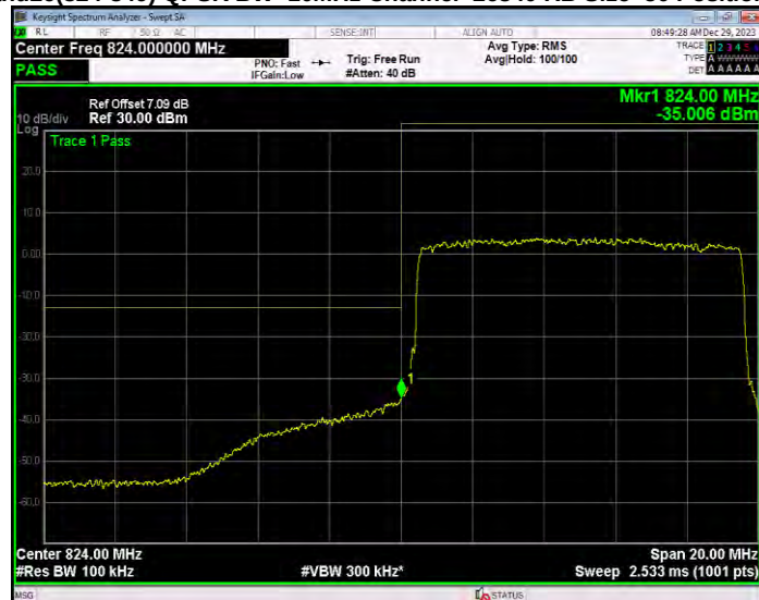
Band26(824-849) QPSK BW=10MHz Channel=26840 RB Size=50 Position=#0
