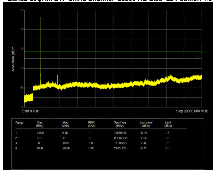
Band2 16QAM BW=3MHz Channel=19185 RB Size=15 Position=#0
