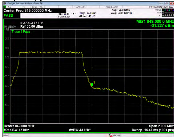
Band26(824-849) QPSK BW=10MHz Channel=26840 RB Size=50 Position=#0
