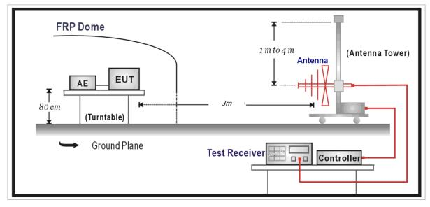
Above 1GHz Test Setup:
