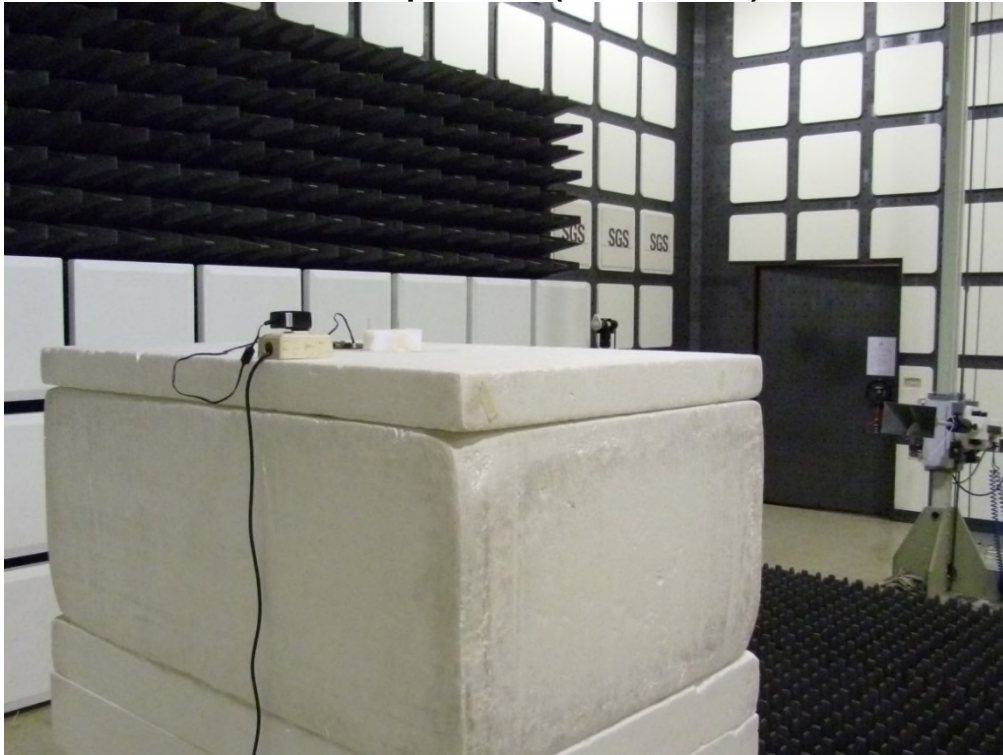
Radiated Emission Set up Photos (Front View) *PCB Antenna
