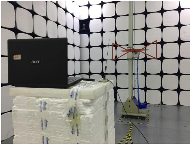
Radiated Spurious Emissions Test Setup Below 1GHz
