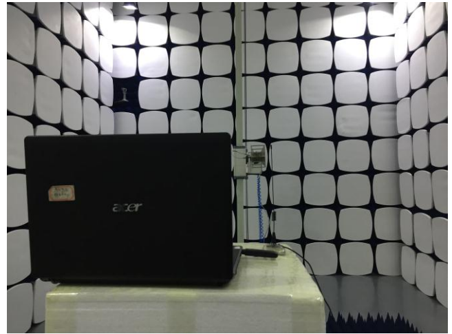
Radiated Spurious Emissions Test Setup Above 1GHz
