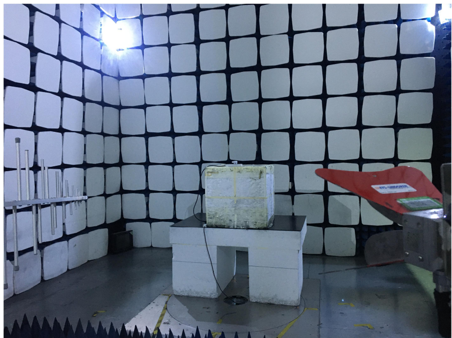
Radiation Emission Test Setup (1GHz to 18GHz)
