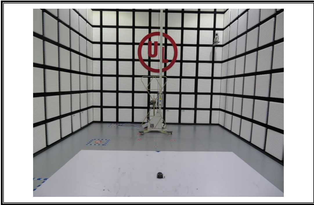
RADIATED RF MEASUREMENT SETUP (30MHz ~ 1 GHz)
