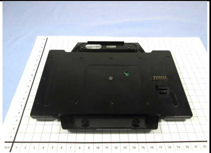
Extended Battery – Rear View
