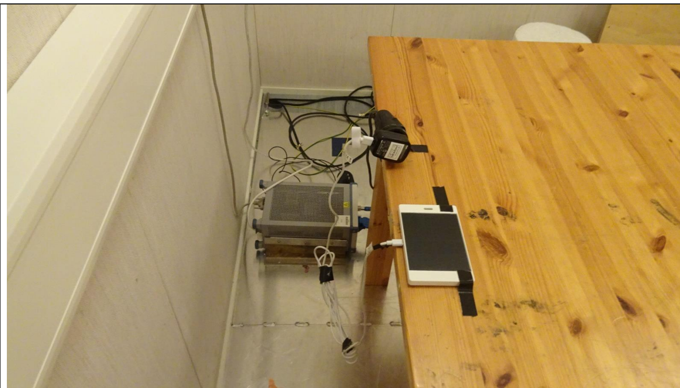
Picture 10, AC Power Line Conducted Emissions
