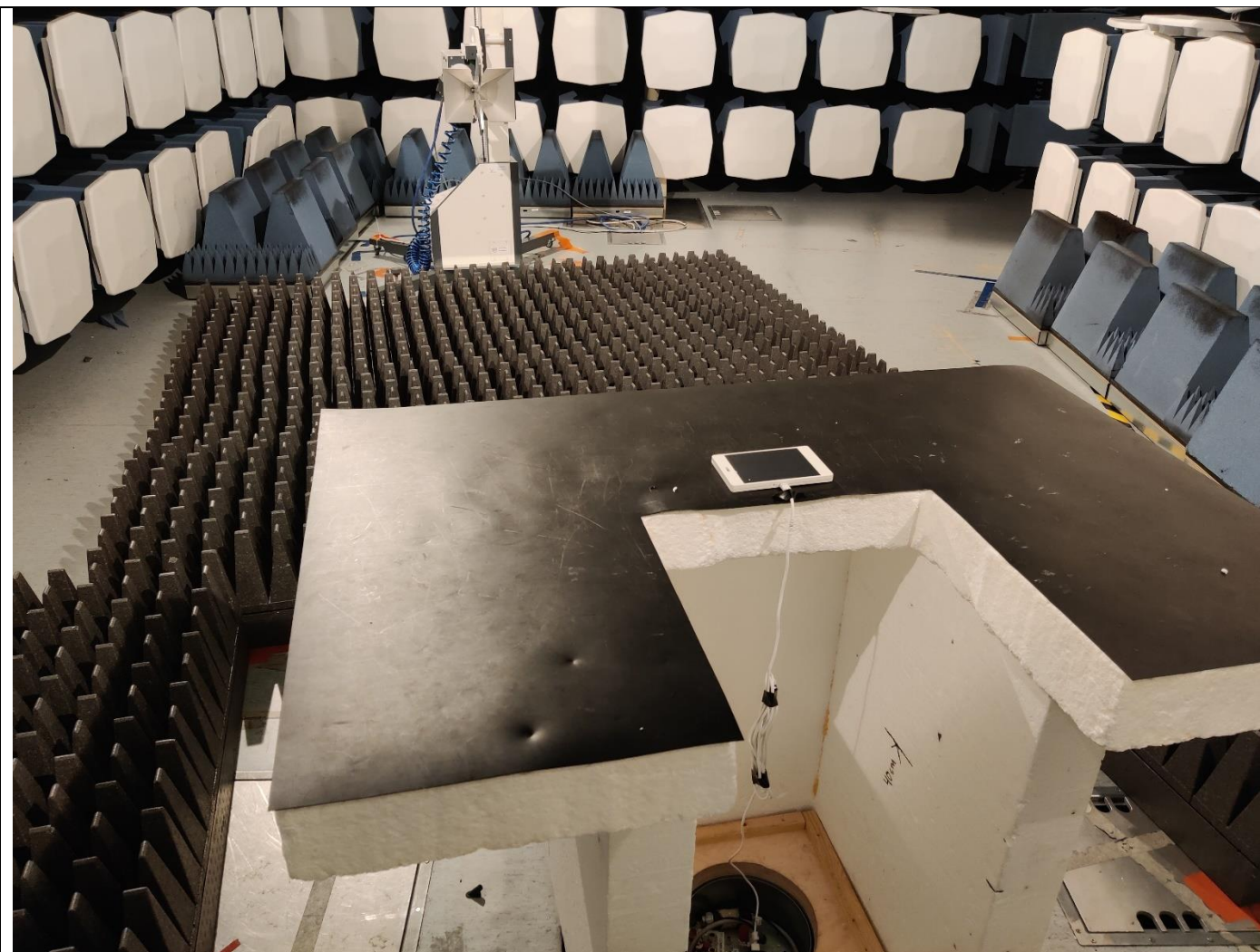
Picture 13, Radiated Spurious Emissions, common setup, RX, 1 – 12,75 MHz
