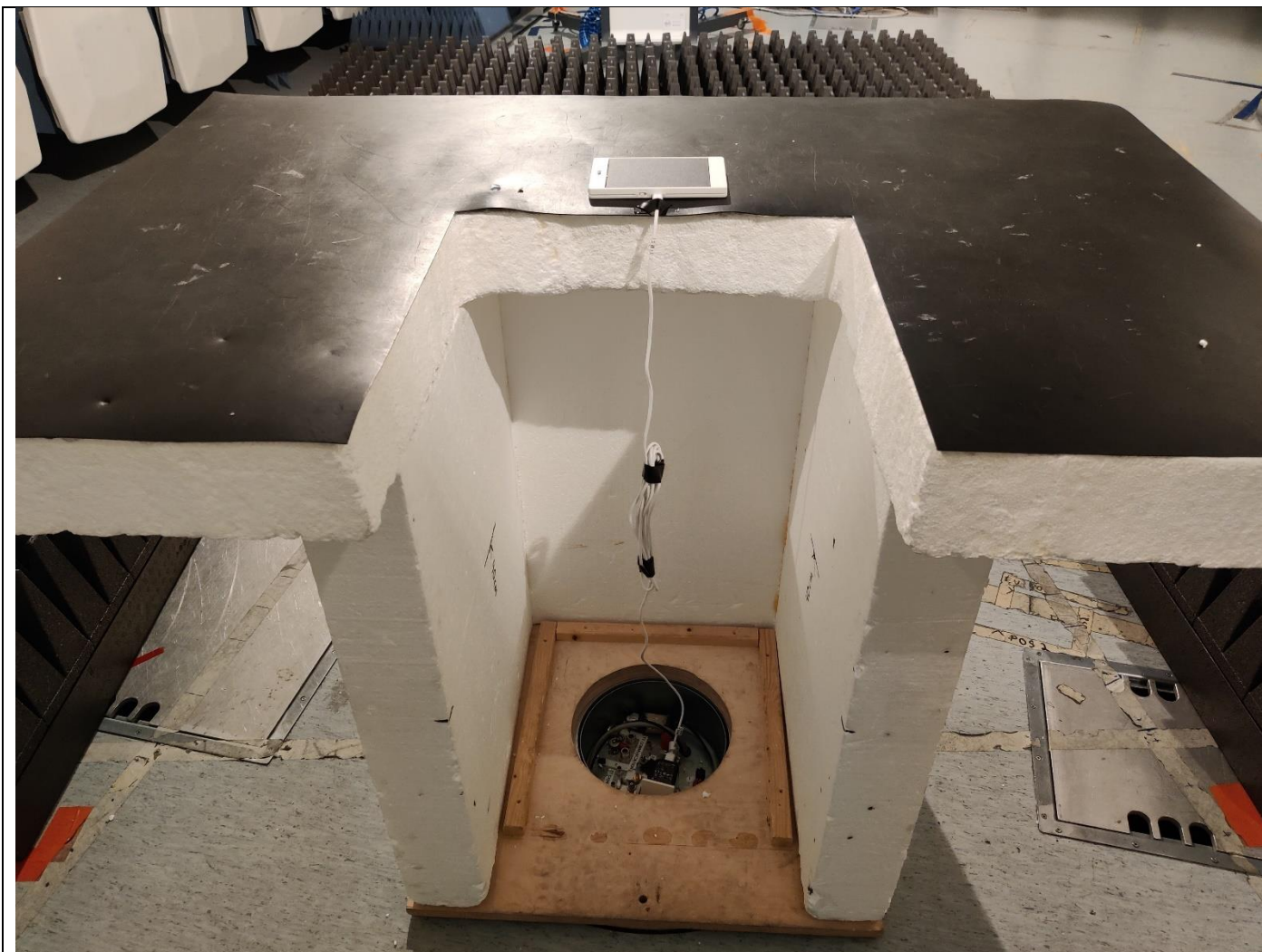
Picture 16, Radiated Spurious Emissions, EUT setup, RX 1 – 12,75 GHz
