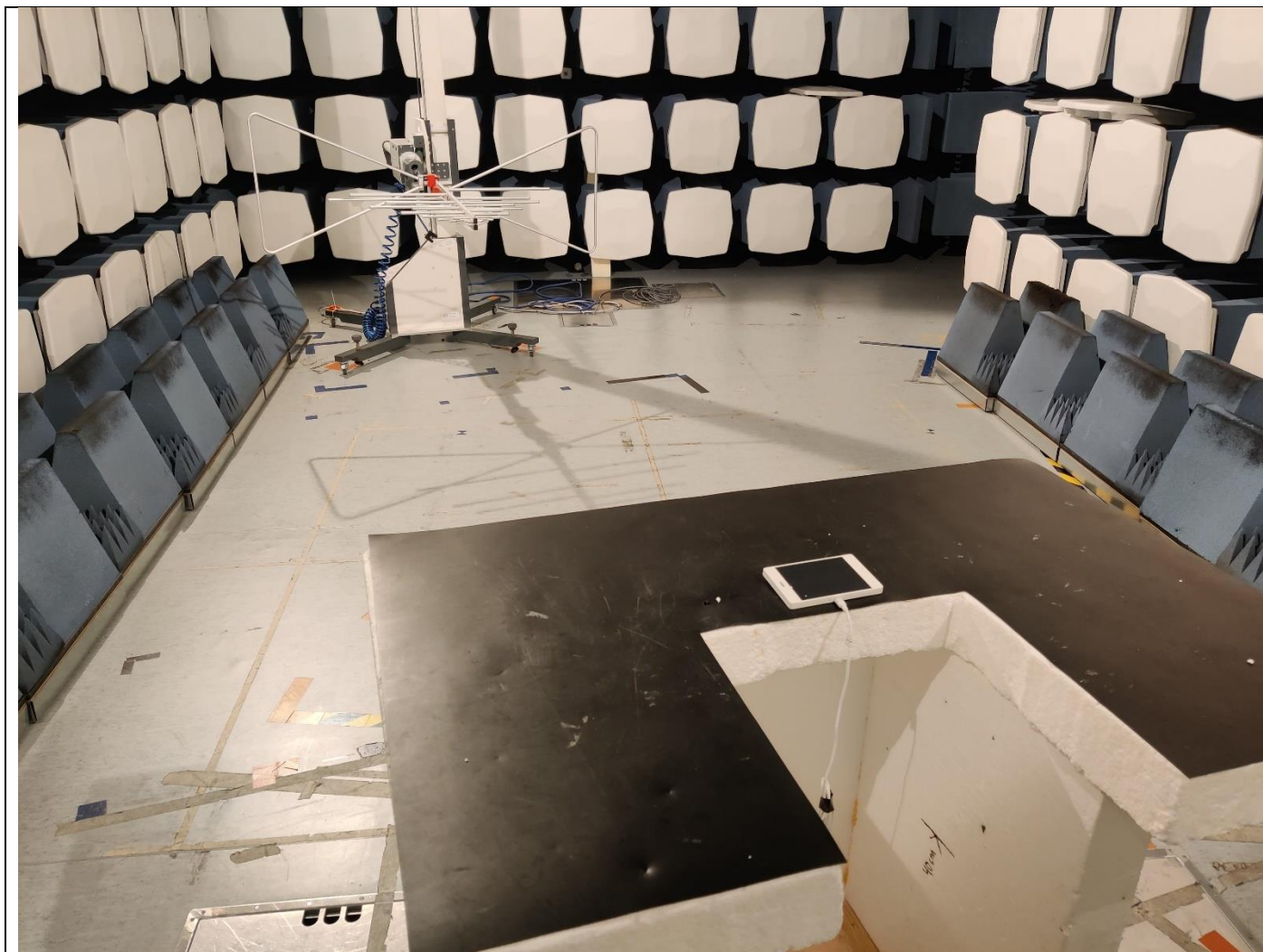
Picture 11, Radiated Spurious Emissions, common setup, TX and RX 30 - 1000 MHz
