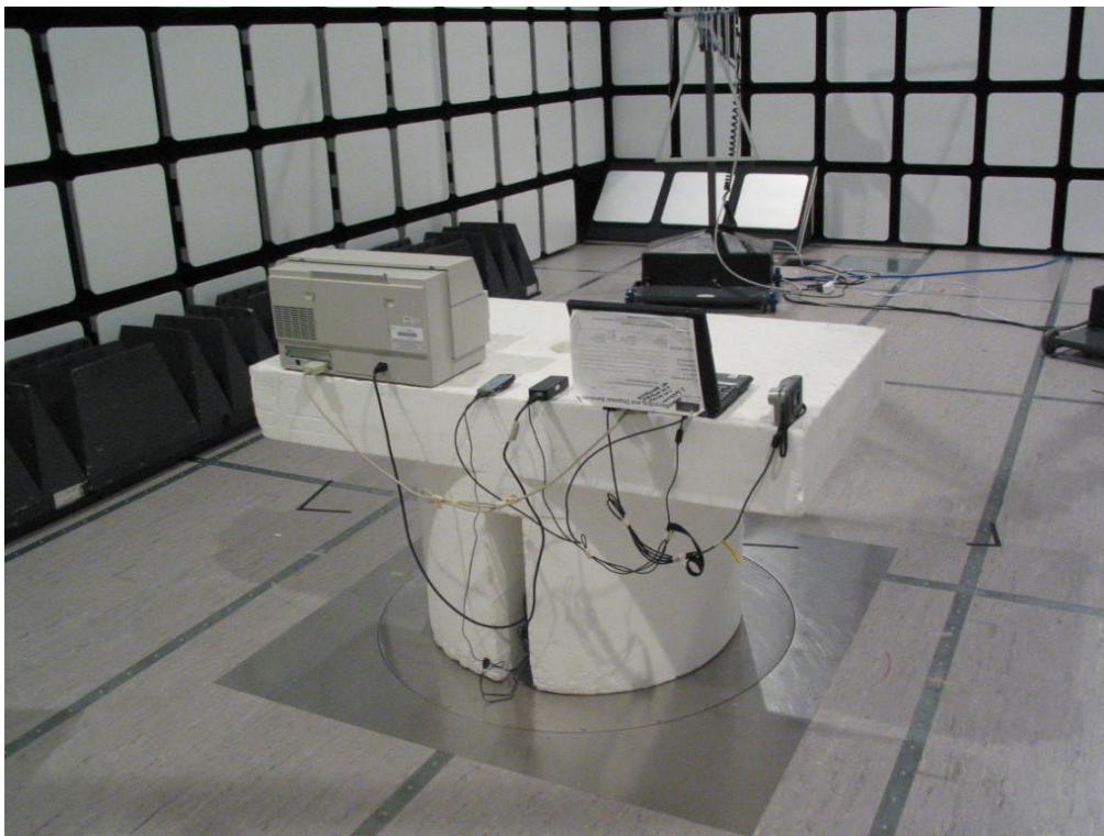
Picture 2 Radiated emission measurement
