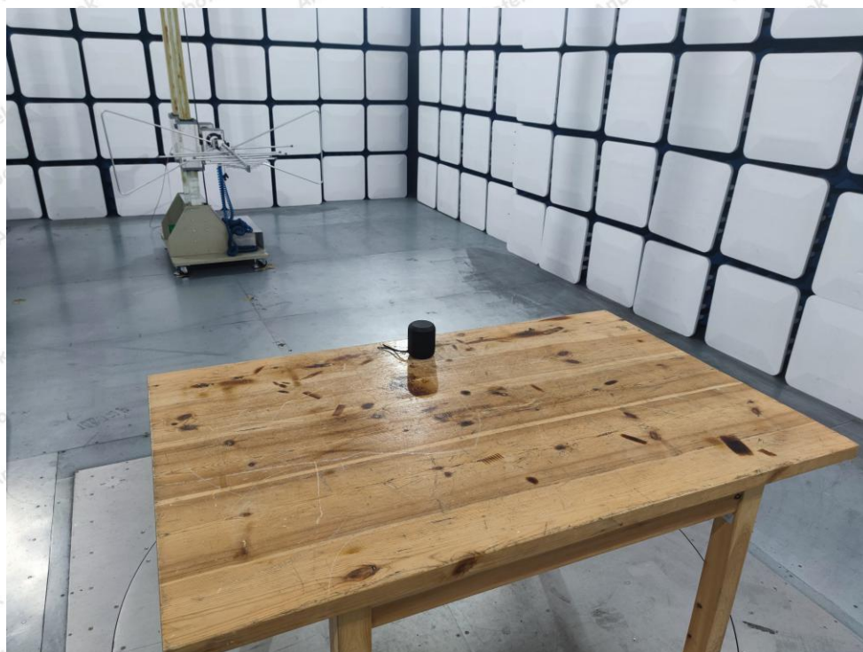
Photo of Radiation Emission Test
