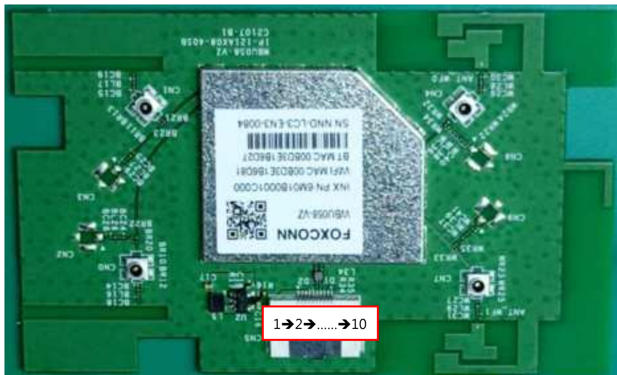
Figure 1 Pin Definitions (Module Top View)
