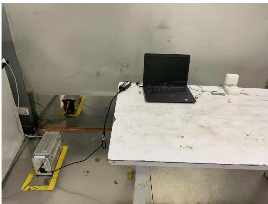
Conducted Emissions Test Setup
