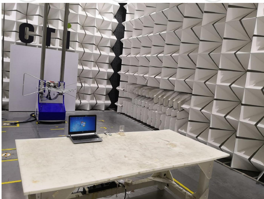
Radiated spurious emission Test Setup-1(Below 1GHz)
