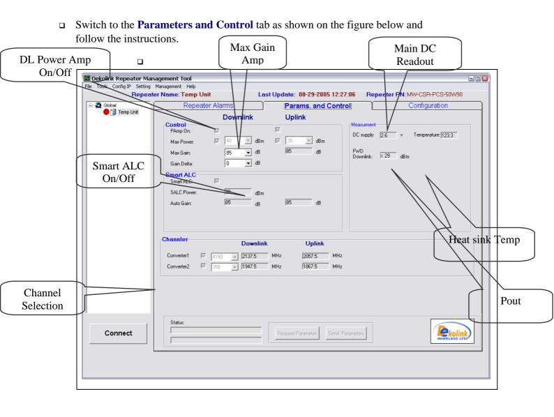
Figure 1: RMS Software - Controls and Parameters Screen
