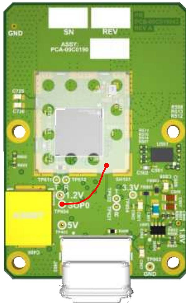
Figure 8. TP604 to Ground Temporary Short
