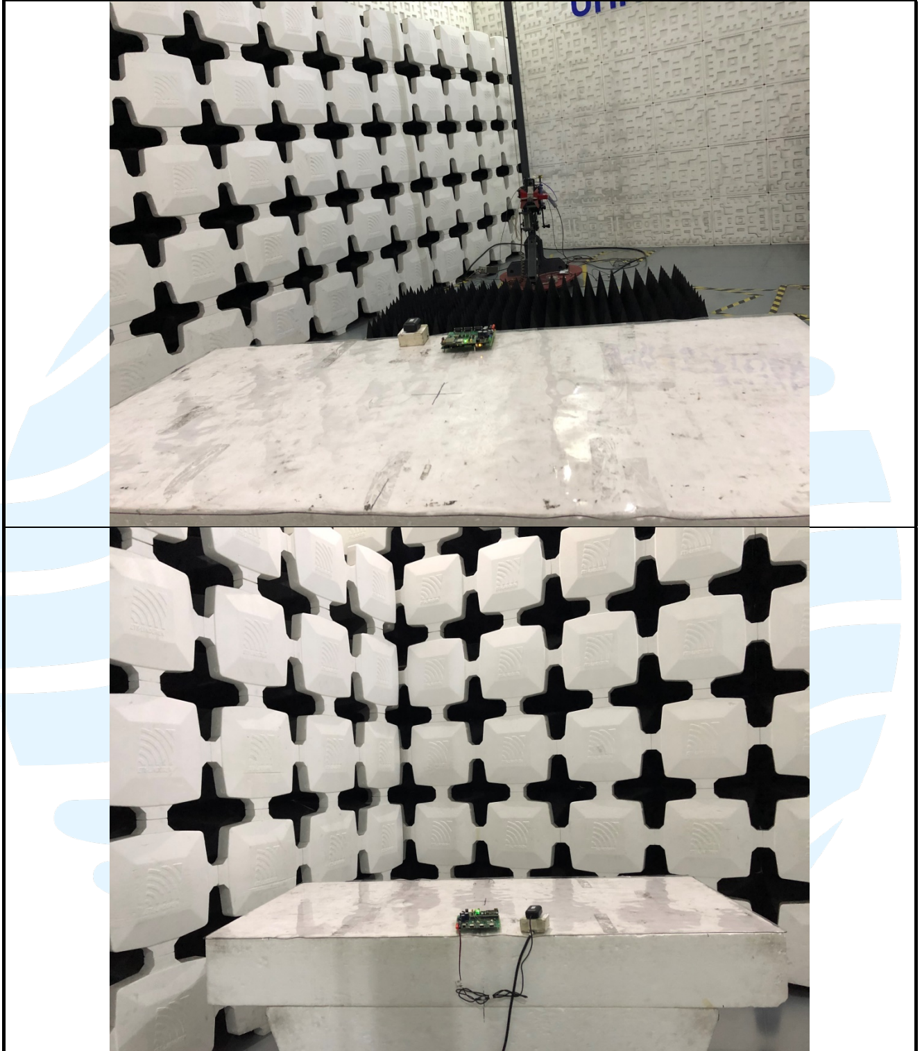
Radiated emission Test Setup-2 (Above 1 GHz)
