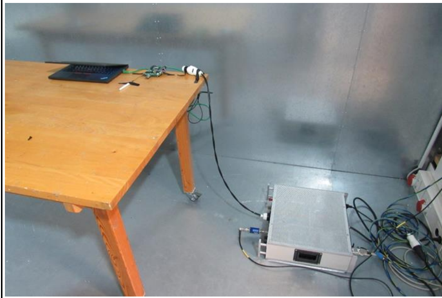
Test setup A - conducted measurement
