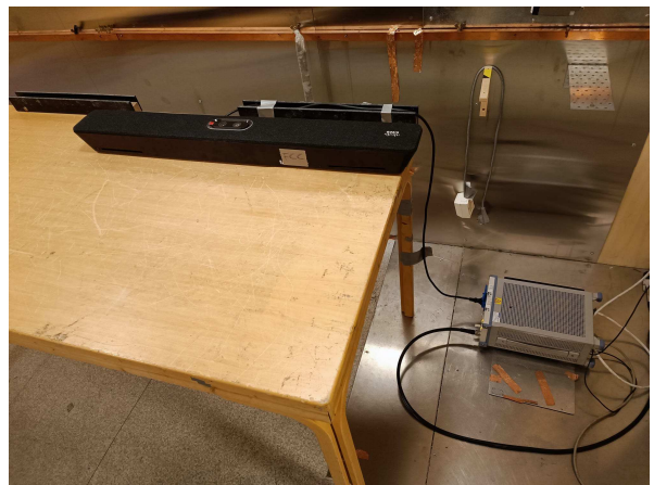
Power-Line Conducted Emissions
